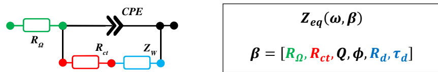
Figure 4.1: Randles model configuration for mixed kinetics and diffusion losses adopted by Fouquet et al. [17], along with associated model parameters.
