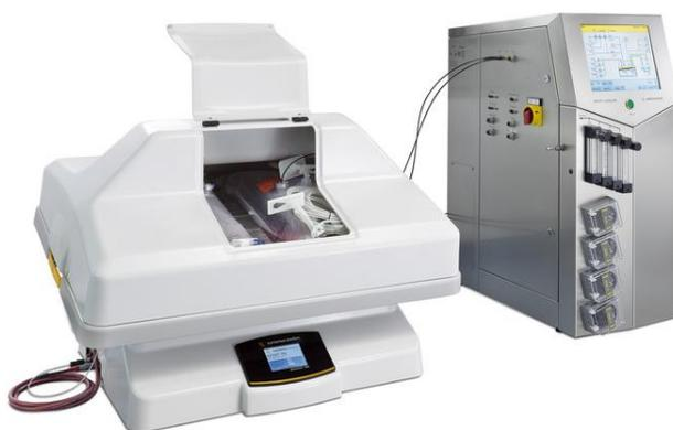
**Figure 11.** The BIostat<sup>®</sup> CultiBag RM Optical provides full process automation with sophisticated feedback control. It consists of a rocker and a digital control unit. The control tower is connected to the rocking unit for monitoring and controlling the culture, including pO<sub>2</sub>, pH, agitation and temperature in batch and fed batch mode operation.
