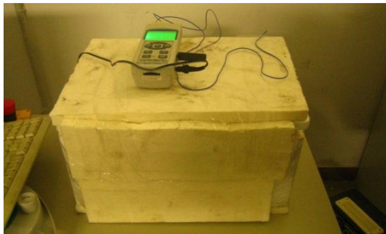
Figure 3.11: Temperature measurement inside insulated mould.
