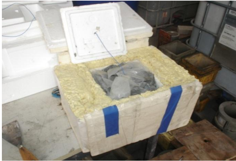
Figure 3.10: Insulated mould inducing semi-adiabatic boundary conditions on the curing concrete sample.
