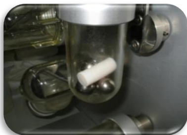
Figure 55: Image of the block of NIP before undergoing the process of grinding in ball mill
