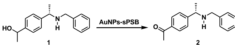
Scheme 4.11: Oxidation of a high molecular weight aminoalcohol.
