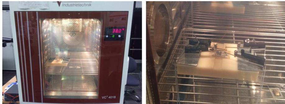
**Figure 3.4** - Votsch climate chamber utilized for Electrical Calcium Test conditionings and measurement station for accommodation of the sample
