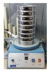
Figure 6.2 Mechanical shaker
