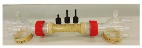
Figure 6.17 Electrokinetic cell
