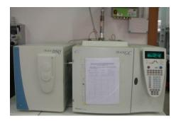
Figure 6.12 GC-MS (Thermofinningan DSQ Trace)
