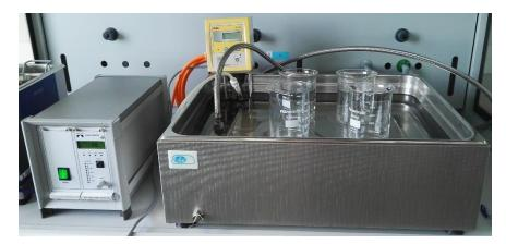
Figure 6.15 Module generators ultrasonic bath (Weber Ultrasonics Sonic Digital MG 1000 TDMF 40-80-120)
