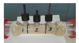
Figure 7.7 Experimental set-up: electrokinetic cell and sample sections
