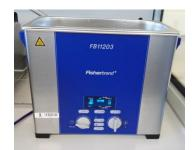
Figure 6.21 Ultrasonic bath (Fisherbrand model FB11203)
