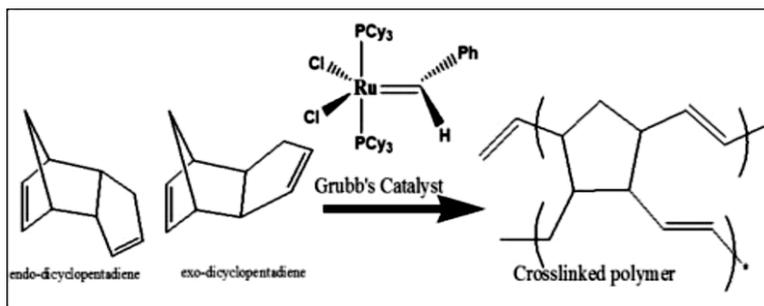
*Figure 1.4:* ROMP reaction of DCPD catalyzed by first generation Grubb's catalyst.
