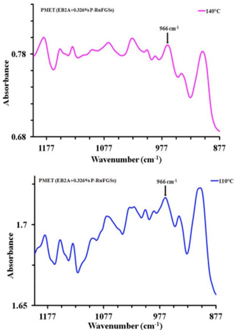
**Figure 2.29:** FT/IR spectra of the solid film (metathesis product) obtained by polymerization of ENB with PolyNBe-GO-HG2 (0.326 wt %) dispersed in the EB2A mixture cured up to 110 °C (graph on the bottom) and cured up to 140 °C (graph on the top).
