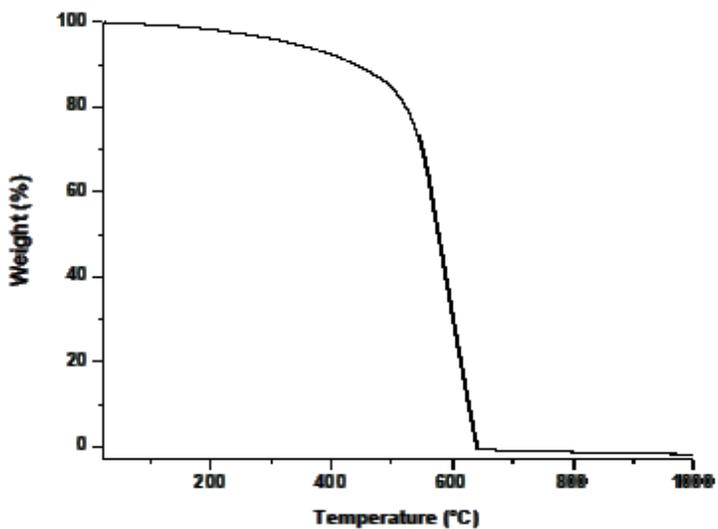
*Figure 2.42:* TGA curve of functionalization MWCNTs with 4-hydroxyphenyl glycine (above) and octyl aldehyde (below).
