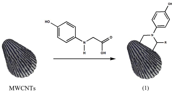
**Figure 2.40:** First step: functionalization of the MWCNTs with 4-hydroxyphenyl glycine and octyl aldehyde.
