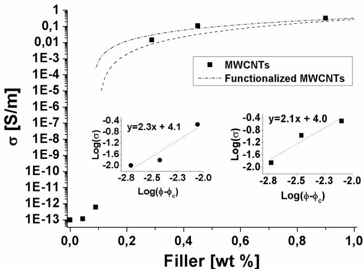
**Figure 3.24:** DC volume conductivity of the nanocomposites versus filler weight percentage. The inserts show the log-log plot of the electrical conductivity as a function of  $(\phi - \phi_c)$  with a linear fit for composites reinforced with pristine and functionalized MWCNTs.
