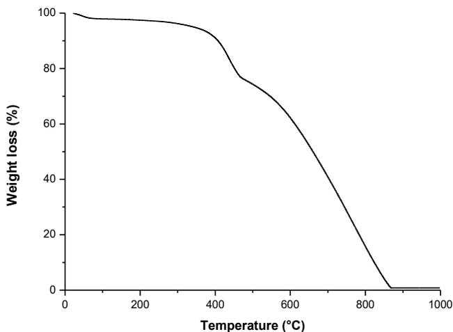
*Figure 3.30:* Thermogram of graphite-pyrene-HG2.
