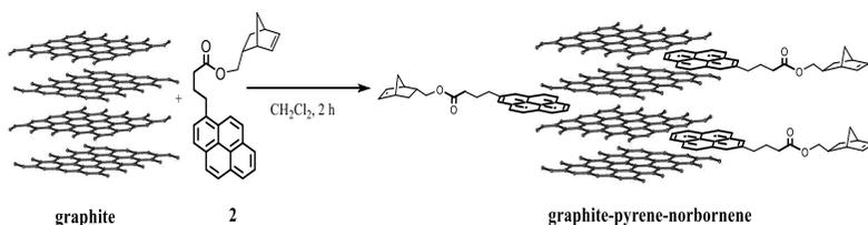
**Figure 3.26:** Functionalization of graphite with pyrene-norbornene.
