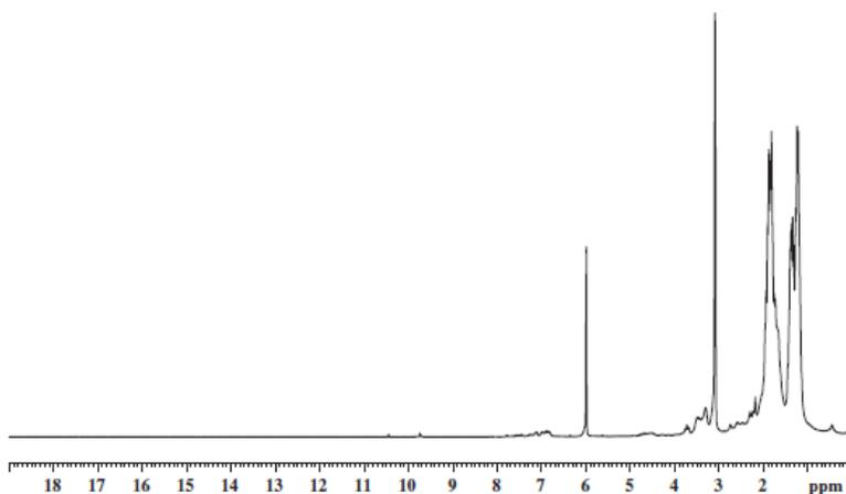
**Figure 2.19:**  $^1\text{H}$  NMR spectra of HG1 and cyclohexene oxide in TCDE kept for 35 min at  $140\text{ }^\circ\text{C}$ .
