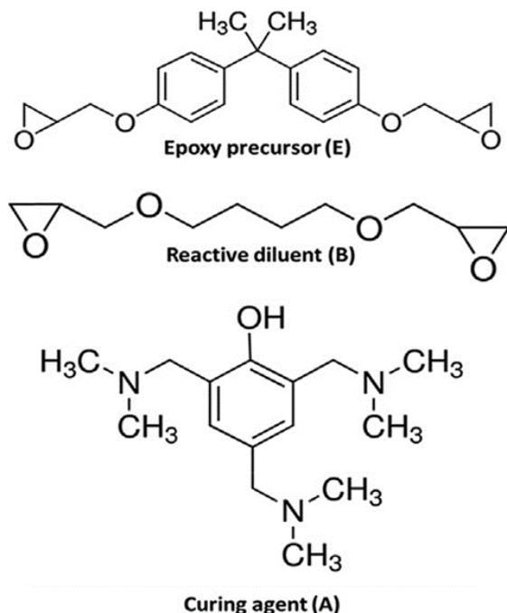
**Figure 2.27:** Chemical formulas of the compounds used for the mixture EB2A.
