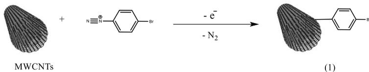
**Figure 2.30:** First step: electrochemical modification of the MWCNTs with 4-bromobenzenediazonium salt.
