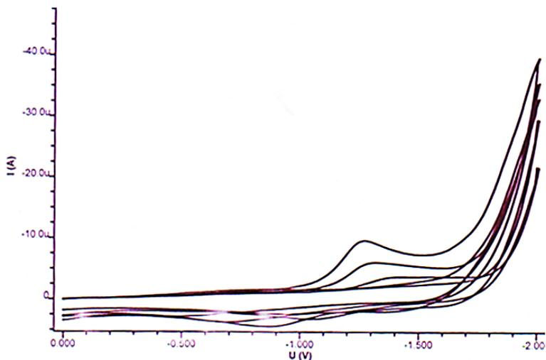
**Figure 2.31:** Voltammogram of electrochemical modification of the MWCNTs with 4-bromobenzenediazonium salt.
