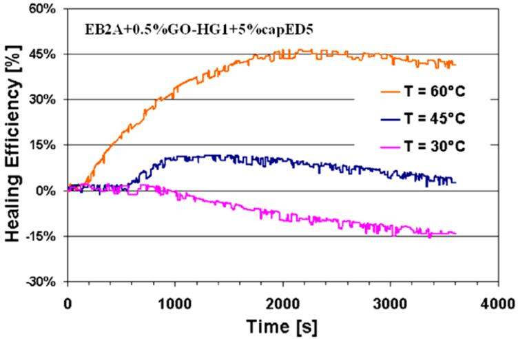
*Figure 2.22:* Time evolution of the relative elastic modulus of the EB2A+0.5%GO-HG1+5% capED5 sample at different temperature.
