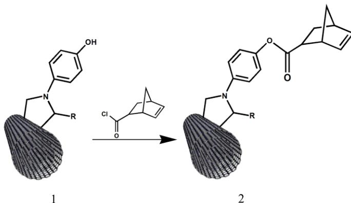
**Figure 2.43:** Functionalization of the MWCNTs with  $\gamma$ -norbornene-2-carbonyl chloride.
