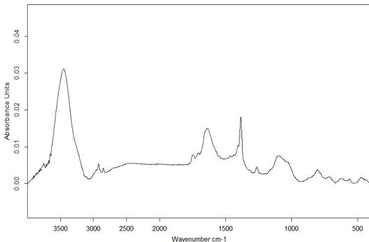
**Figure 2.41:** Spectrum FT/IR of functionalization MWCNTs with 4-hydroxyphenyl glycine and octyl aldehyde.
