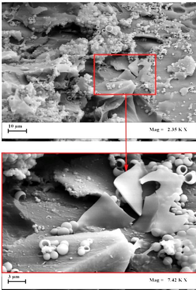
**Figure 2.26:** FESEM images of the globular shell around the catalyst sites attached on graphene sheet (PolyNBE-GO-HG2sample).
