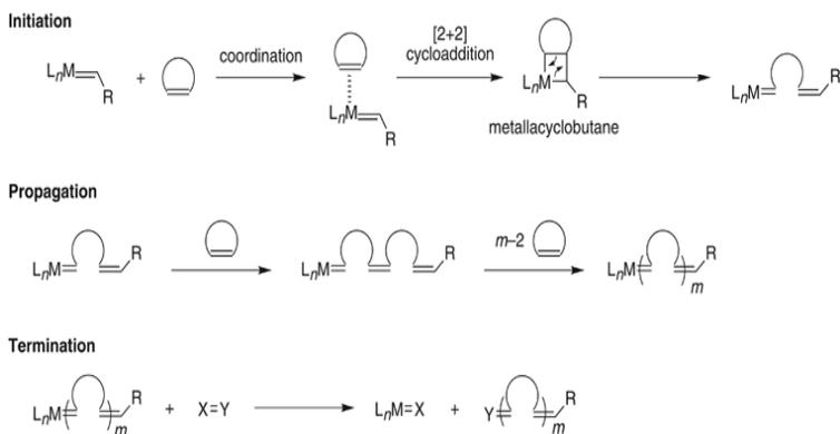
**Figure 1.7:** Mechanism of ROMP reaction.
