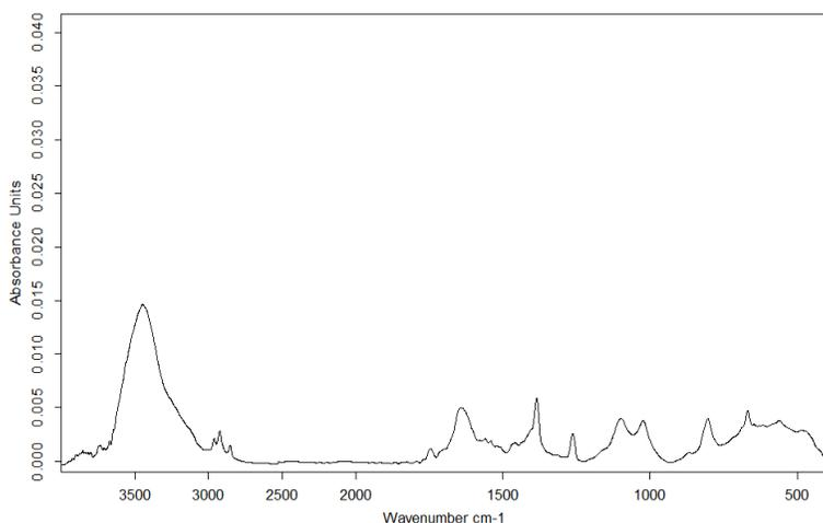
**Figure 2.48:** Spectrum FT/IR of functionalization of graphite with 4-hydroxyphenyl glycine and octyl aldehyde.
