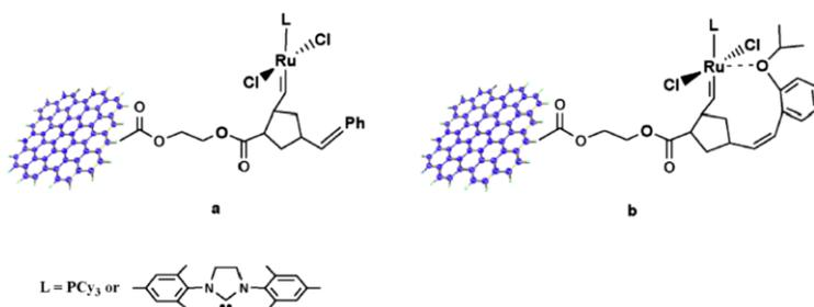
**Figure 2.16:** Possible structure of G1 and G2 (a) and HG1 and HG2 (b) ruthenium catalysts after reactions to chemically bind them to GO.
