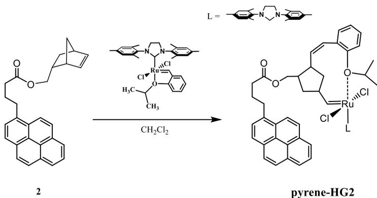
**Figure 3.16:** Metathesis reaction that bind the Hoveyda Grubbs II generation catalyst to the pyrene.
