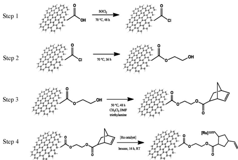
**Scheme 2.2:** Functionalization of GO with Ru-based catalysts.
