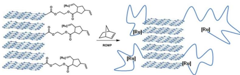
**Figure 2.24:** Scheme of the reaction for the protection of catalyst.
