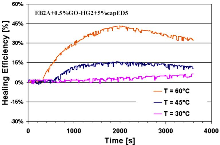
*Figure 2.23:* Time evolution of the relative elastic modulus of the EB2A+0.5%GO-HG2+5% capED5 sample at different temperature.
