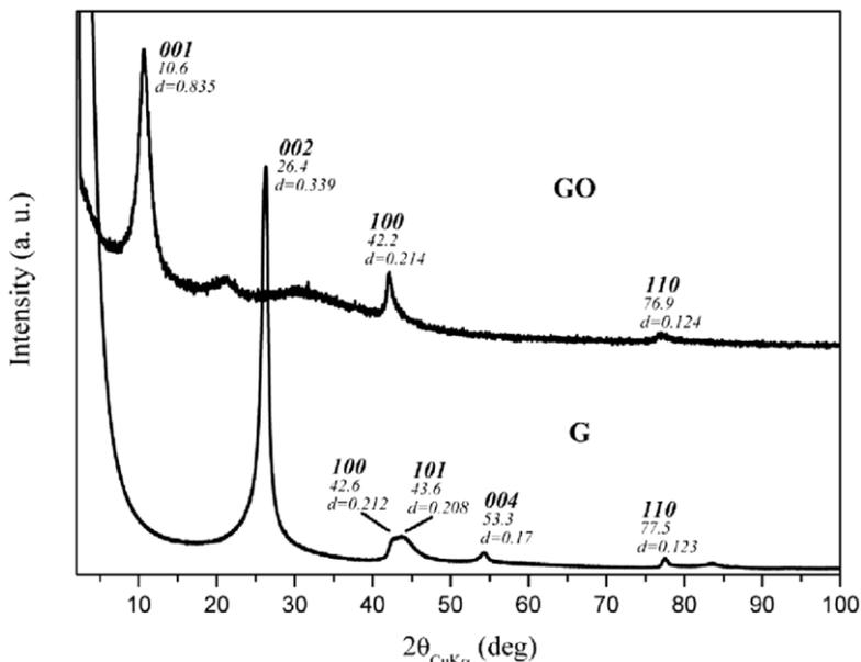
**Figure 2.8:** X-ray diffraction patterns (Cu K $\alpha$ ) of the starting high surface area graphite (G) and of graphene oxide (GO).
