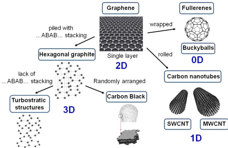
*Figure 1.14:* All graphitic allotropes.
