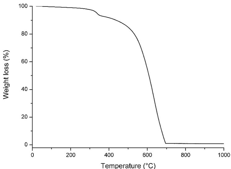
**Figure 3.2183:** Thermogram in air at 1000 °C of MWCNTs-pyrene-G1.
