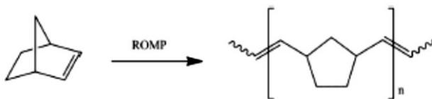
*Scheme 2.3:* Ring Opening Metathesis Polymerization of 2-norbornene.
