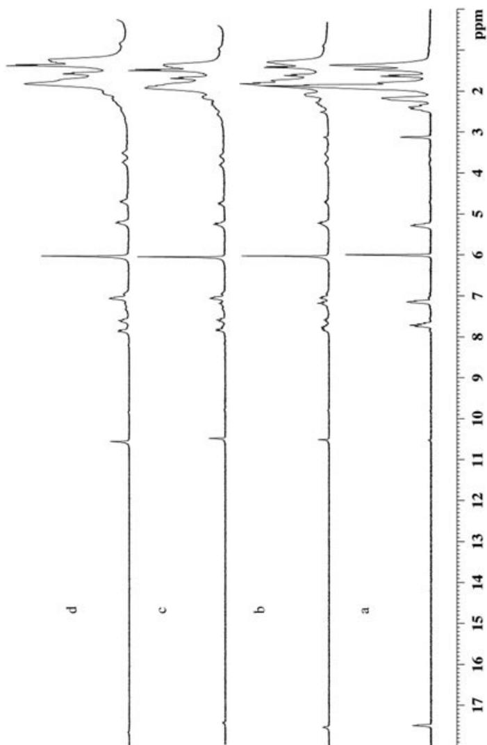
**Figure 10.18:** VT  $^1\text{H}$  NMR experiments on a mixture containing HG1 and cyclohexene oxide in a molar ratio 1:1 ((a) 80 °C, (b) 100 °C, (c) 120 °C, and (d) 140 °C).
