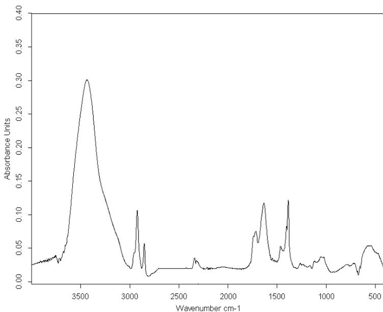
**Figure 2.39:** Spectrum FT/IR of MWCNTs.
