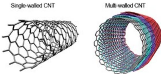
**Figure 1.17:** Structure of Single Walled Carbon Nanotubes (SWCNTs) and Multi Walled Carbon Nanotubes (MWCNTs).
