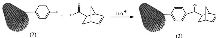
**Figure 2.35:** Third step: functionalization of the MWCNTs with 5-norbornene-2-carboxaldehyde.
