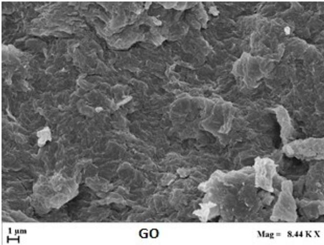
*Figure 2.5:* FESEM pictures of graphite (G) and graphene oxide (GO).
