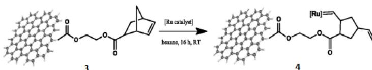
*Figure 2.12:* Metathesis reaction with Ru-based catalyst.
