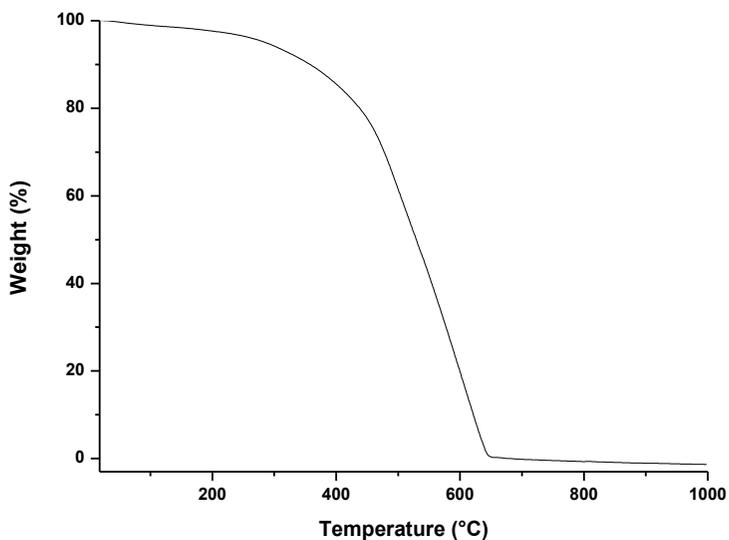
*Figure 2.49:* TGA curve of functionalization of graphite with 4-hydroxyphenyl glycine and octyl aldehyde.
