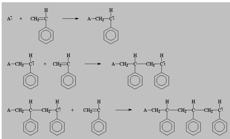
**Figure 4.3:** Schematic representation of the reaction of polymerization of the styrene ( $A\cdot$  is the initiator).
