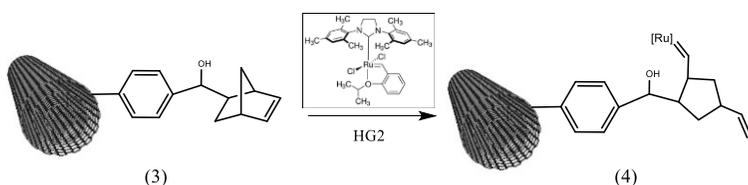
**Figure 2.36:** Fourth step: functionalization of the MWCNTs with Ru-based catalyst.
