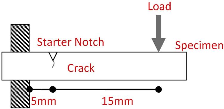
*Figure 25:* Test geometry adapted for the healing tests.
