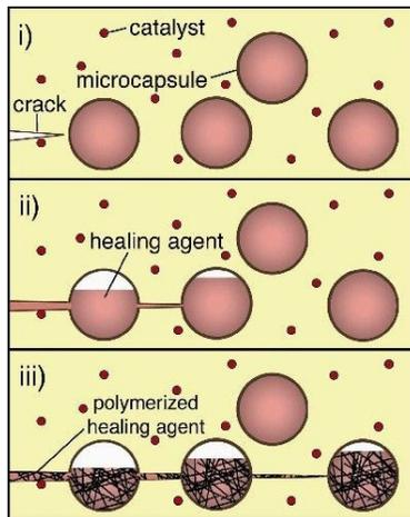
**Figure 1.1:** Step of the repairing mechanism that begins after a fractures.
