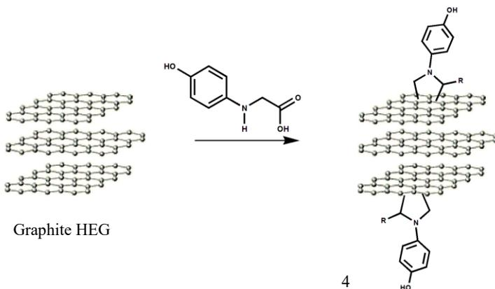
**Figure 2.47:** First step: functionalization of the graphite with 4-hydroxyphenyl glycine and octyl aldehyde.
