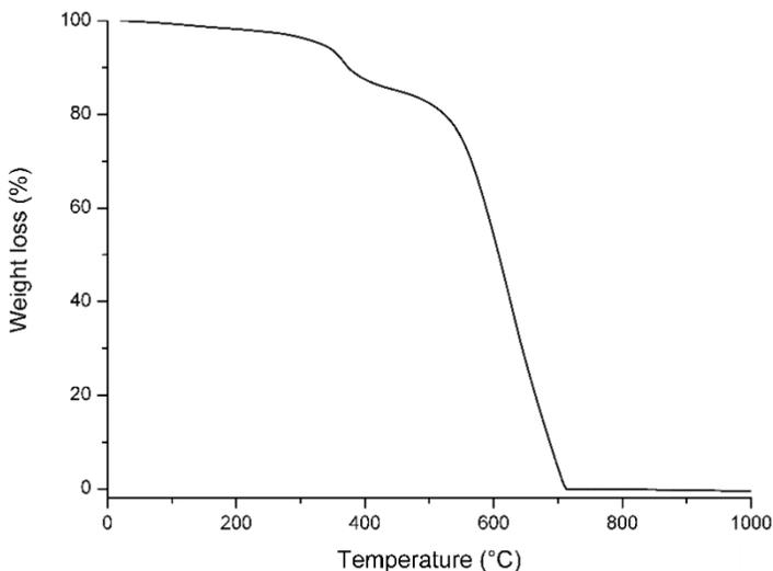
**Figure 3.20:** Thermogram in air at 1000 °C of MWCNTs-pyrene-HG2.
