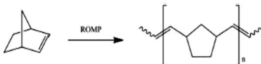
*Scheme 3.1:* Ring Opening Metathesis Polymerization of 2-norbornene.
