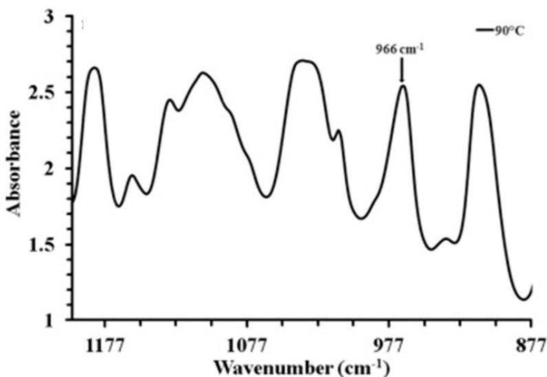
**Figure 2.28:** FT/IR spectrum of the solid film (metathesis product) obtained by polymerization of ENB with PolyNBe-GO-HG2 (0.326 wt %) dispersed in the EB2 mixture at 90 °C.
