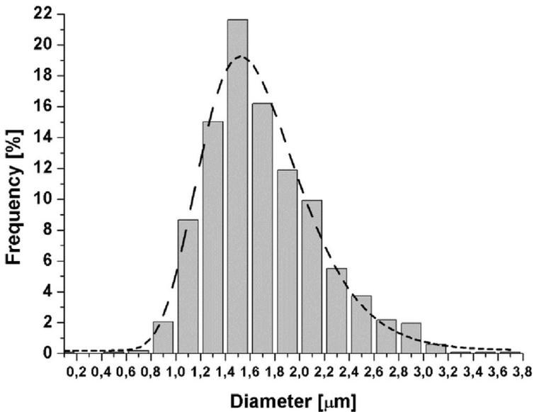
*Figure 2.21:* Histogram of the microcapsule diameter.
