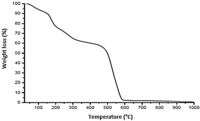
*Figure 2.7:* Thermogram of GO in air.
