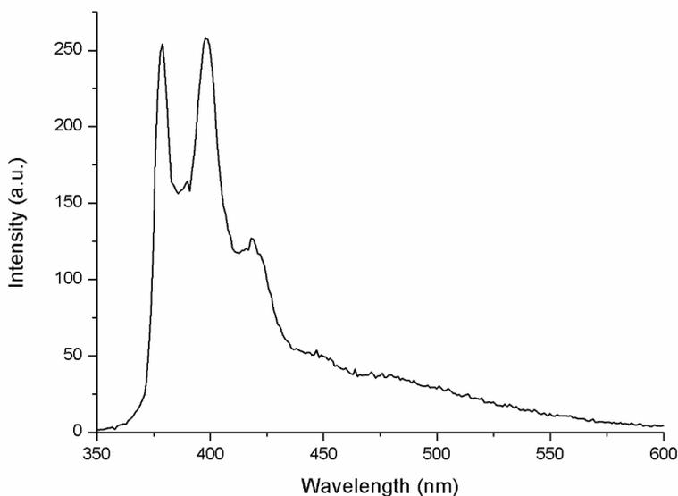
**Figure 3.25:** Fluorescence spectra of soluble fraction MWCNTs-pyrene in boiling decaline.
