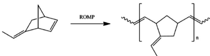
*Scheme 3.2:* Ring Opening Metathesis Polymerization of 5-ethyliden-2-norbornene.
