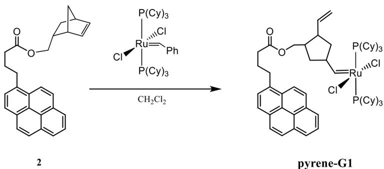
**Figure 3.17:** Metathesis reaction that bind the Grubbs I generation catalyst to the pyrene.
