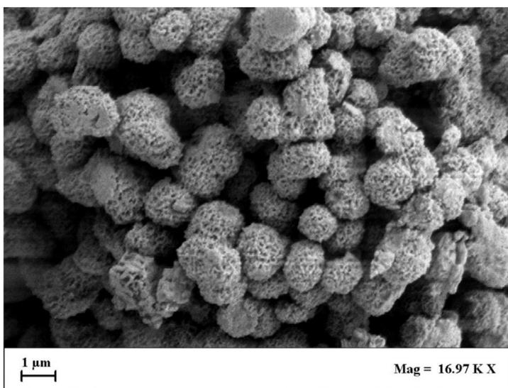
**Figure 2.20:** FESEM image of the microcapsules (capED5) in the form of spherical snarls.
