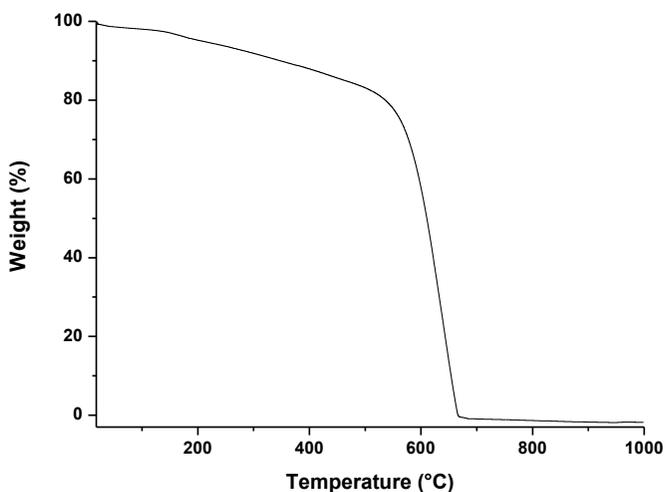
Figure 2.44: TGA curve of functionalization MWCNTs (2).
