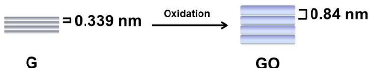
**Scheme 2.1:** Schematic representation of the increasing of the interlayer distance in GO after oxidation of graphite G.
