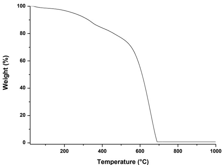
*Figure 2.46:* TGA curve of functionalization MWCNTs (3).
