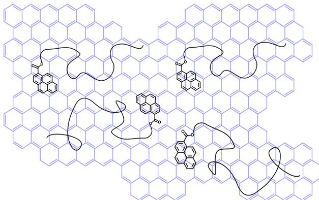
**Figure 3.21:** graphitic plane with a polymer-pyrene linked by  $\pi$  - stacking interaction.
