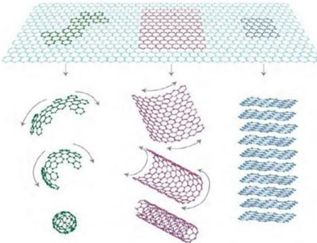
**Figure 1.15:** Schematic representation of graphene, which is the fundamental starting material for a variety of fullerene materials; buckyballs, carbon nanotubes, and graphite.
