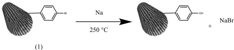
**Figure 2.32:** The alkaline fusion of MWCNTs-Ph-Br.
