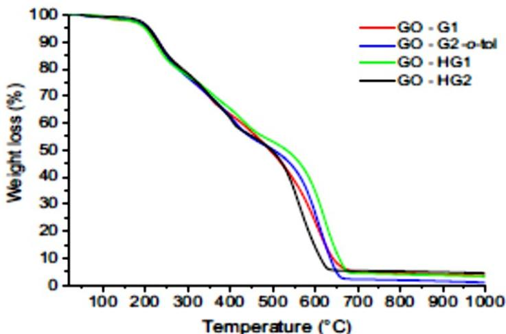
*Figure 2.13:* Thermogram in air at 1000 °C of the Ru-based catalysts covalently bonded to the GO.
