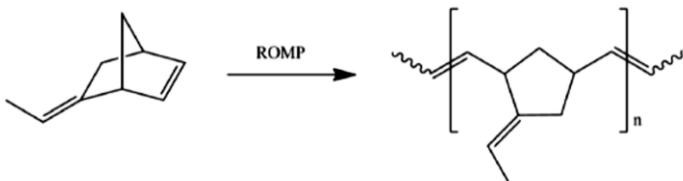
**Scheme 2.4:** Ring Opening Metathesis Polymerization of 5-ethyliden-2-norbornene.
