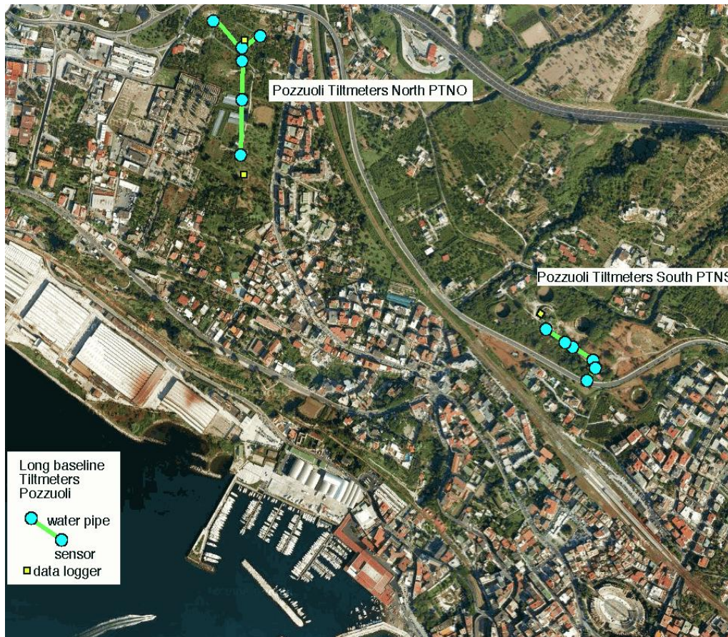
Figure 3.15 – Placement of the two instruments in respect with the Pozzuoli town, and their current length. Instruments are in scale.
