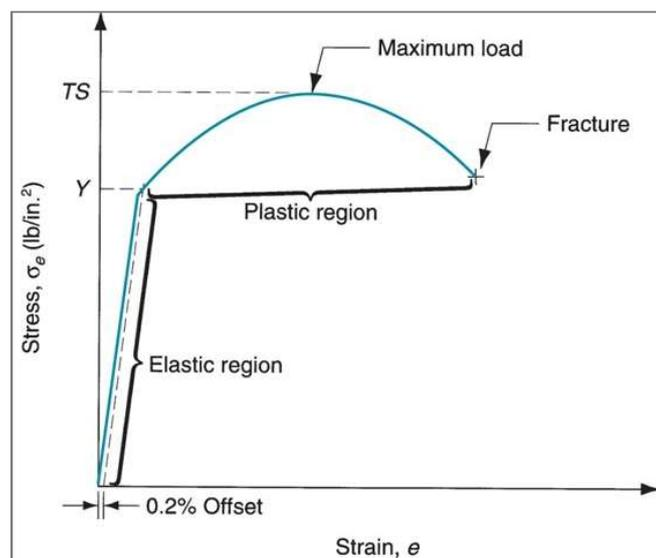
**Figure 50.** Typical Stress-Strain Plot
