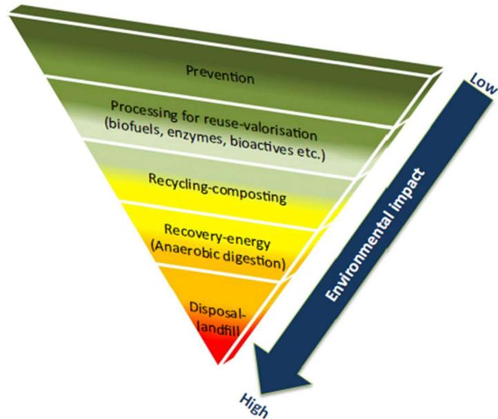
**Figure 3.** Hierarchy for waste processing (Ravindran and Jaiswal, 2016)
