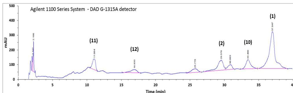
**Figure 15.** HPLC-DAD fingerprint (230 nm) of hazelnut shells extract (HSE). The peak numbers in this figure correspond to compounds in **Figure 14**.
