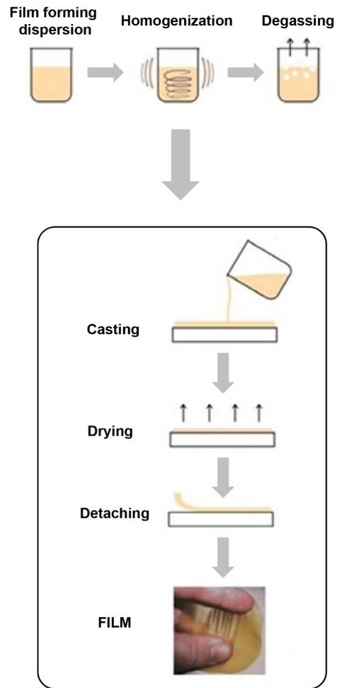
**Figure 12.** Production of films by casting technique (Otoni et al., 2017)
