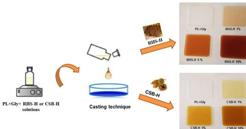
Figure 47. Films preparation by Casting technique
