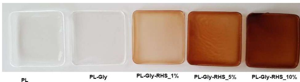
**Figure 36.** Photographs (by digital camera CANON EOS 600D) of films loaded with RHS-H (composition in **Table 15**)
