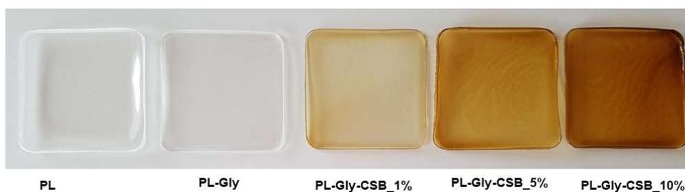
**Figure 37.** Photographs (by digital camera CANON EOS 600D) of films loaded with CSB-H (composition in **Table 15**)
