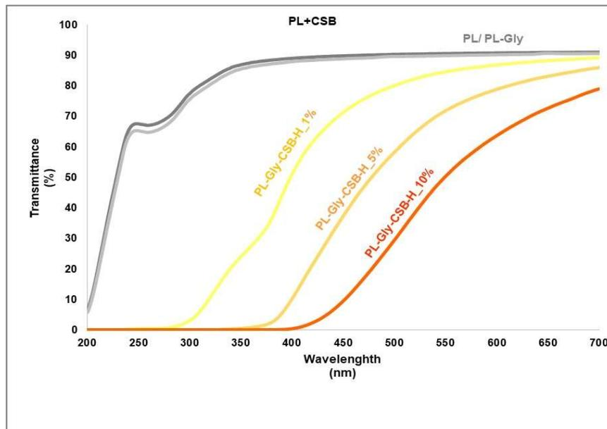
**Figure 39.** UV-vis spectra of blank (PL; PL-Gly) and CSB-H-loaded films
