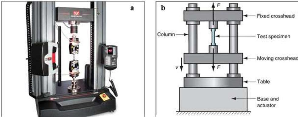
**Figures 49. (a)** Instron 5966 Series machine and **(b)** operating mechanism
