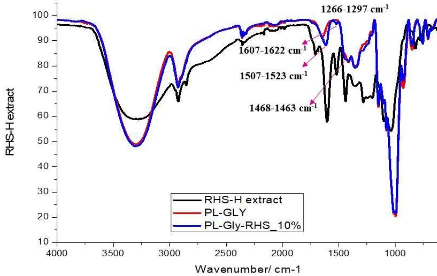
**Figure 42.** FTIR spectra of raw extract (RHS-H black line), blank film (PL-Gly, red line) and loaded film (PL-Gly-RHS-H\_10%, blue line)
