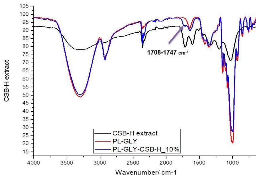
**Figure 43.** FTIR spectra of raw extract (CSB-H black line), blank film (PL-Gly, red line) and loaded film (PL-Gly-CSB-H\_10%, blue line)
