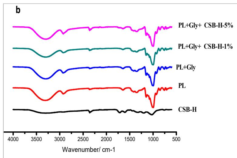
**Figure 41.** FTIR spectra of raw extracts (**a** RHS-H and **b** CSB-H), blank films (**a** and **b** PL and PL-Gly) and loaded film (PL-Gly-RHS-H\_1%, PL-Gly-RHS-H\_5%, **Figure a**; PL-Gly-CSB-H\_1%, PL-Gly-CSB-H\_5%, **Figure b**)
