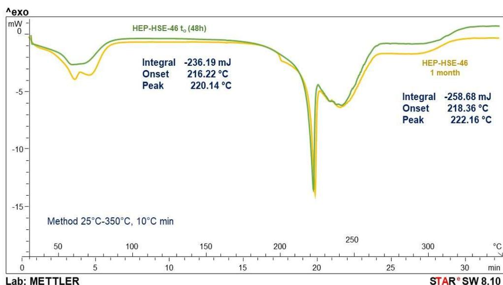
**Figure 27.** Differential scanning calorimetry (DSC) thermograms of HEP-HSE46 at  $t_0$  (green profile), and after 1 month (yellow line)
