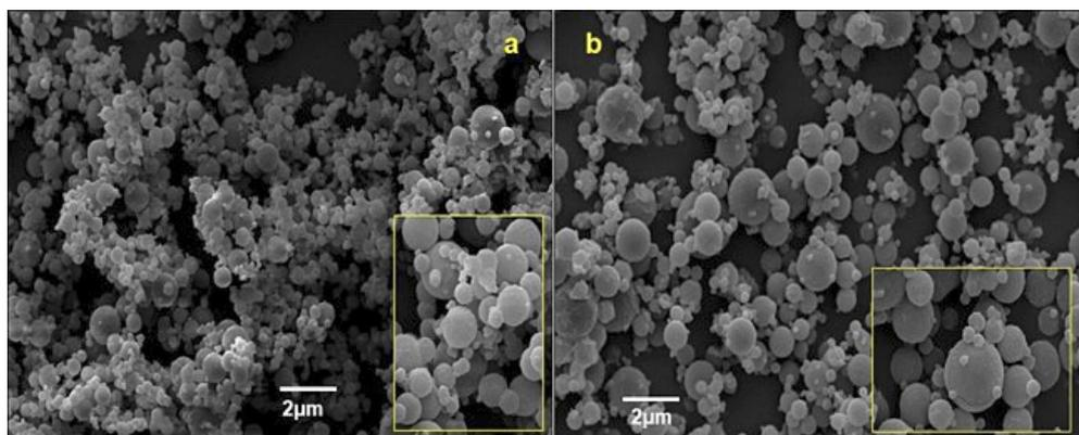
**Figure 30.** Scanning electron microscopy (SEM) images of (a) HEP-HSE-46 at  $t_0$  and (b) HEP-HSE-46 after 6 months
