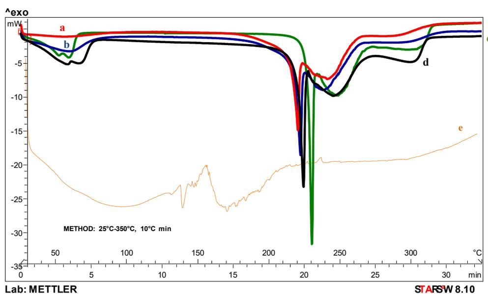
**Figure 25.** Differential scanning calorimetry (DSC) of HEP-HSE-46 (a), HEP-46 (b), HEP-1 (c), HEP-HSE (d) and compared to unprocessed extract (HSE, e).
