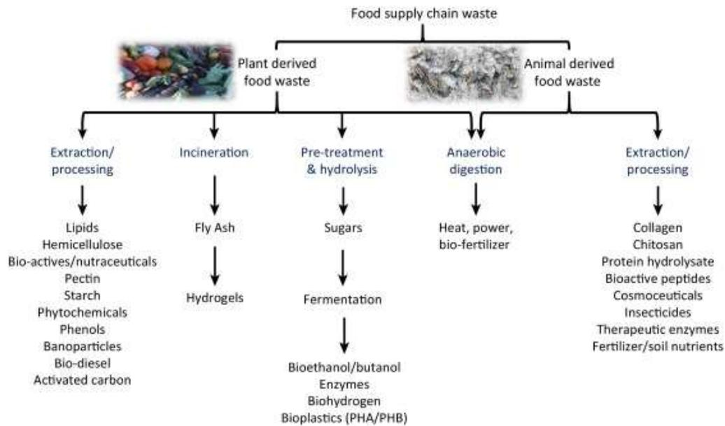
**Figure 4.** Flow diagram of reutilization of wastes (Ravindran and Jaiswal, 2016)
