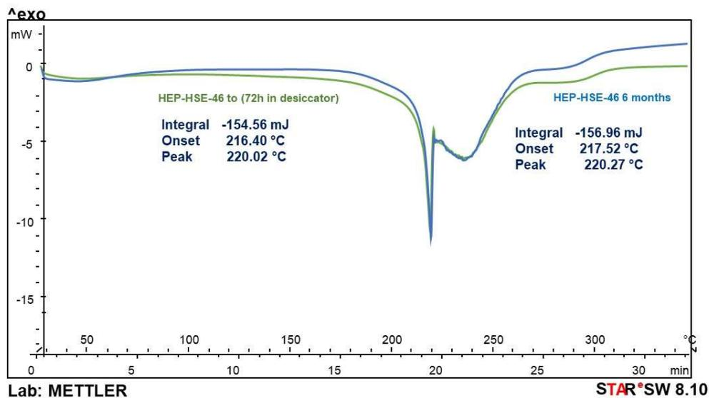
**Figure 29.** Differential scanning calorimetry (DSC) thermograms of HEP-HSE-46 at  $t_0$  (green profile), and after 6 months (blue line)
