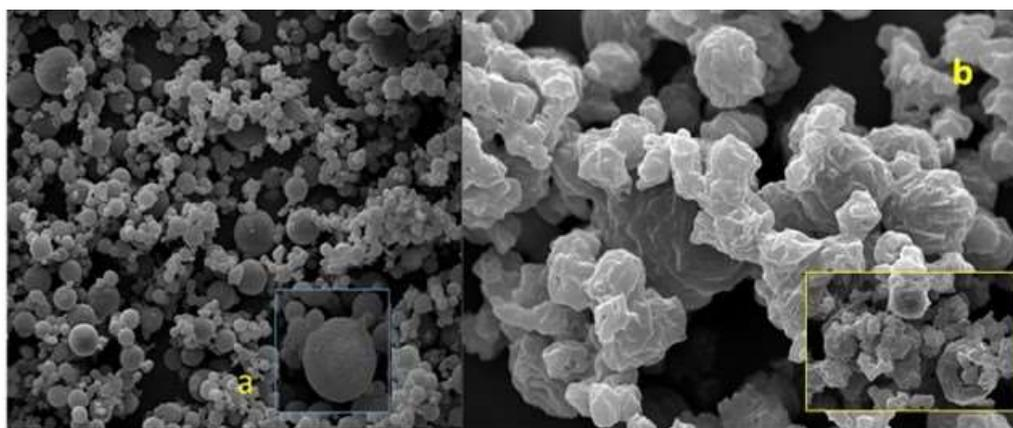
**Figure 28.** Scanning electron microscopy (SEM) images of (a) HEP-HSE-46 at  $t_0$  and (b) HEP-HSE-46 after 1 month
