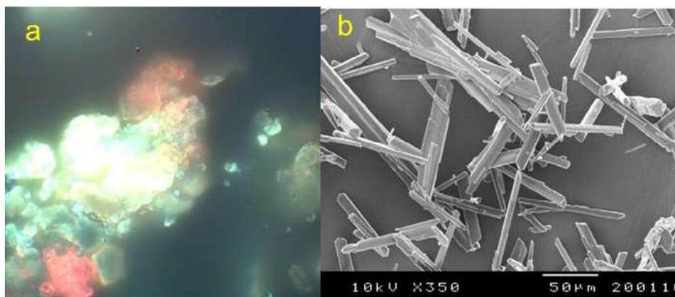
**Figure 21.** FM image (a) of HSE raw material and SEM micrographs (b) of L-proline (reported by Hyung et al., 2008): crystalline clusters with difference fluorescence (a) due to the different nature of bioactive compounds
