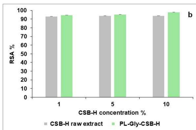
**Figure 44.** DPPH scavenging activity of RHS-H raw extract and PL/RHS-H films (**a**) and CSB-H raw extract and PL-Gly-CSB-H films; values are the mean of three independent experiments; error bars represent the standard deviation
