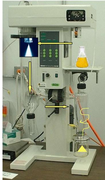
**Figure 8.** Spray drying process
