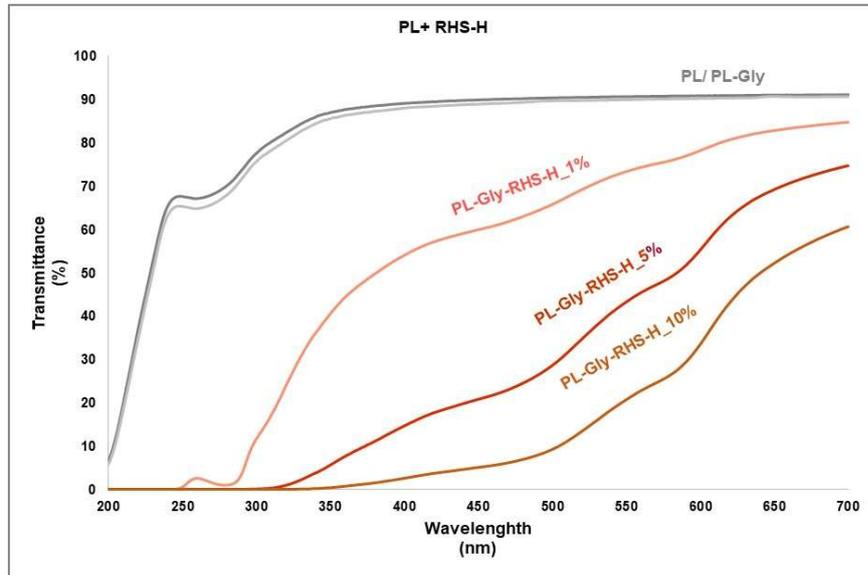
**Figure 38.** UV-vis spectra of blank (PL; PL-Gly) and RHS-H-loaded films
