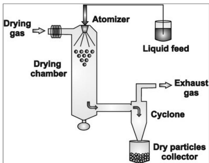
**Figure 7.** Diagram of the equipment and process of conventional spray-drying (Sosnik and Seremeta, 2015)
