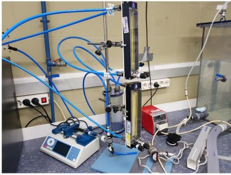
Figure 7-9: Synthetic gas stream generation system
