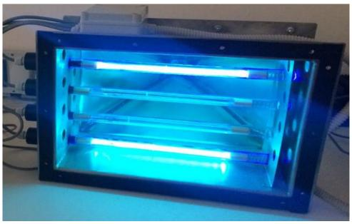
Figure 7-3: UV lamps configuration
