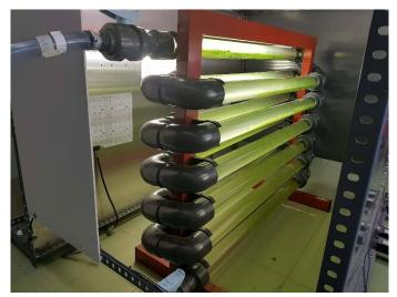
Figure 7-7: Tubular Photo-Bioreactor
