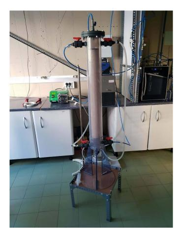
Figure 7-6: Biotrickling filter
