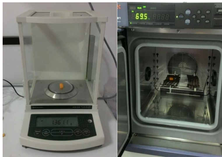
Figure 37 Digital balance (Shimadzu mod. AW320) and bench-top temperature humidity chamber (Espec Corp. mod. SU-221).
