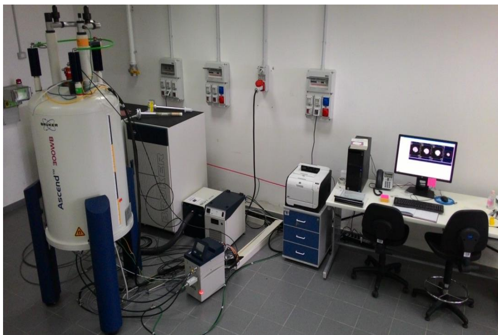
Figure 27 Magnet, Operator Console, and Console at MNR Laboratory of Physics Department of Salerno.
