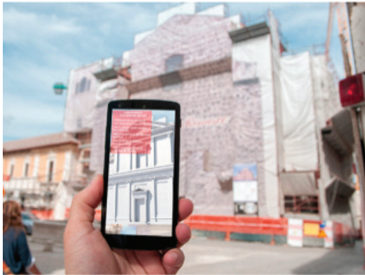
Fig. 1 -Application of Augmented Reality with the virtual reconstruction of the unbuilt facade of Santa Margherita Church in L'Aquila. The model, linked to a two-dimensional target, can be visualized in real time. The test app was created using Unity 3D and the augmented reality plugin Vuforia ( https://www.vuforia.com/ ) (Brusaporci, Ruggieri, Sicuranza, Maiezza, 2017, p.9).
