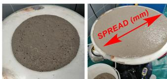
**Figure 22.** Slump test for the studies of the dosage-dependent effect of the synthesized macrocycles **1** and **2** on mortar spread value (bottom) and
