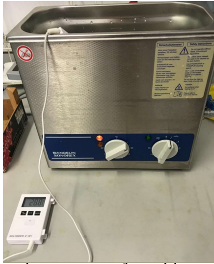
Figure III.7 Ultrasound pre-treatment of pear slabs
