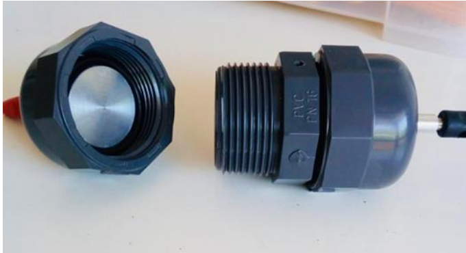
Figure 4.10 Cylindrical treatment cell
