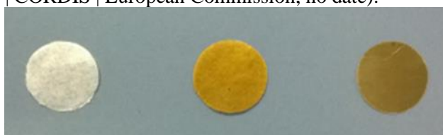
Figure 8 Photographs of bioplastic made by tomato cuticle during the BIOPROTO project
