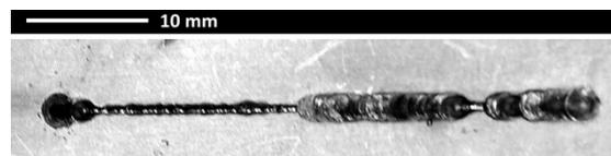
FIGURE 6.4 – BOP test sample: no key-hole development below the threshold irradiance
