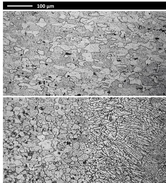
FIGURE 6.15 – AA 2024 T3, micrograph: base metal (above) and HAZ at the bead interface (below)
