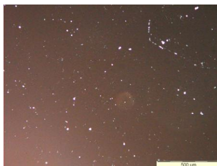
Figure VIII.8 Optical image of T20BD+5%GPOSS sample after ultrasonication and magnetic stirring in oil bath at 120°C for 1h
