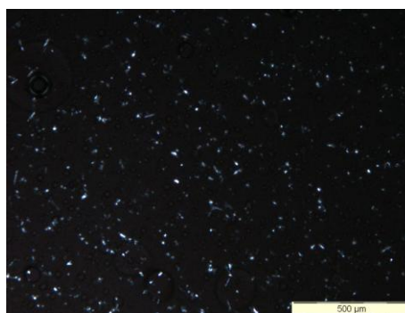
Figure VIII.9 Optical image of T20BD+5%TCPOSS sample after ultrasonication and magnetic stirring in oil bath at 120°C for 1h
