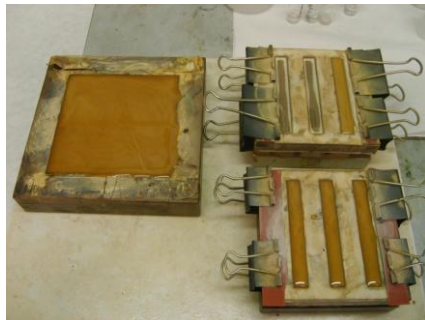
Figure IX.29 BAMPO based uncured epoxy mixture poured into molds used for fire testing
