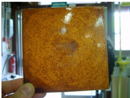
Figure IX.33 Tested epoxy sample containing BAPPO particles homogeneously dispersed
