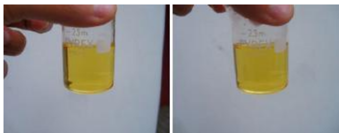
Figure VIII.5 Photos of T20BD+5%ECPOSS mixture after ultrasonication (on the left) and after 1h in a stirred oil bath at 120°C (on the right)
