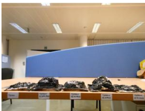
Figure VIII.12 Photographs of residues from left to right (neat T20BD, T20BD+5%DPHPOSS, T20BD+5%ECPOSS, T20BD+5%GPOSS, T20BD+5%TCPOSS)
