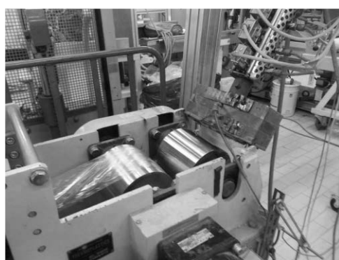
Fig. IV.2 Extrusion of the Active PET Film with the lab-scale extruder (THERMOPLASTICS Tokyo-Japan).
