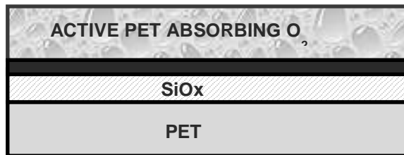
FIGURE IV.8. Scheme of the multilayer structure for the solar cell barrier encapsulant
