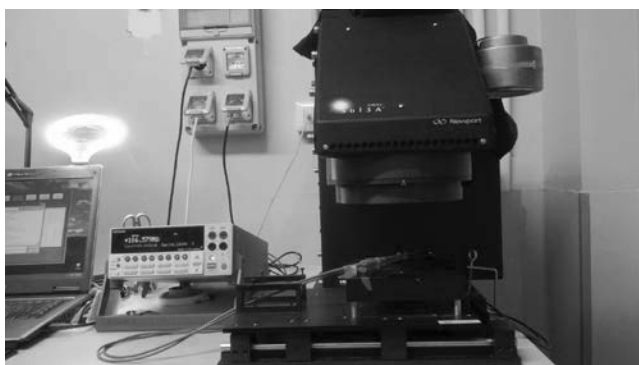
Figure V.5 I-V measurement for encapsulated solar cell exposed to solar simulator
