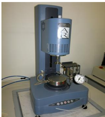
Figure 4.2. Rheometer used for tests with plate and cone geometry TA Instruments AR 2000 (TA Instruments, New Castle, DE).
