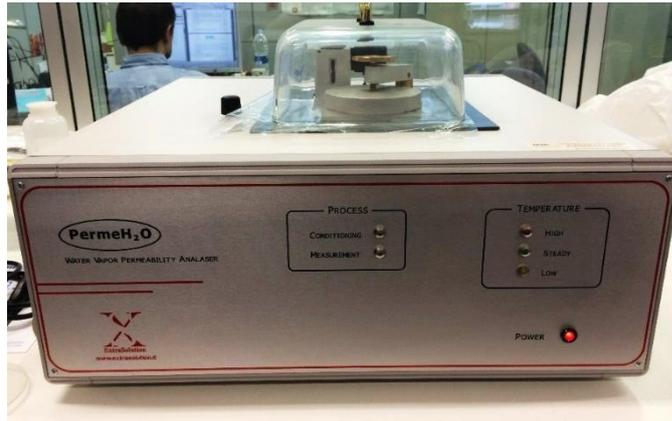
**Figure 5.2** - PermeoH<sub>2</sub>O permeabilimeter by ExtraSolution for WVTR barrier film measurement.
