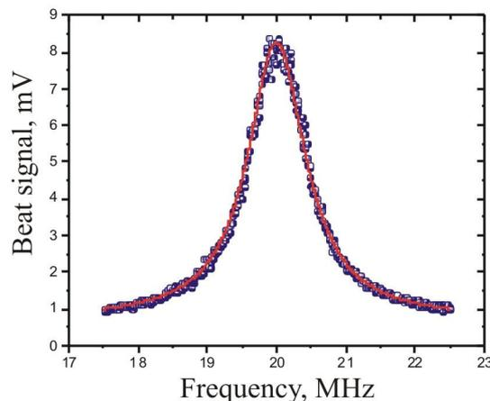
Fig. 2.5.2.3. Example of a beat note signal between DFB-DL and closest in frequency component of the optical frequency comb under lock conditions.
