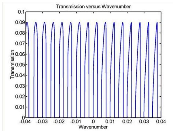
Fig. 2.5.1.3. Transmission signal of the V-cavity.
