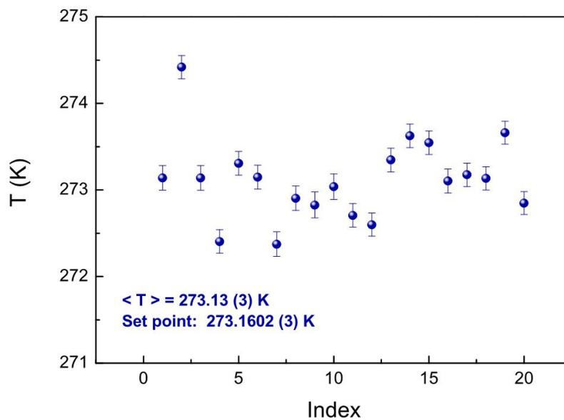
Fig. 4.4.1. Spectroscopic determinations of the gas temperature. Each point results from the global fitting of four spectra recorded at different pressures.
