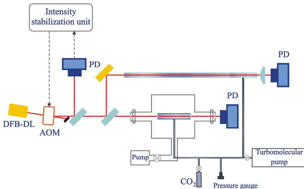
Fig. 3.2.2.1. Sketch of the experimental setup used for absorption cell length determination. DFB-DL stands for distributed feedback diode laser, AOM - acousto-optic modulator, PD - photodetector.
