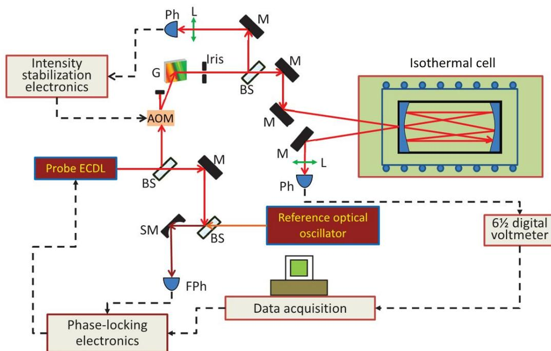
Fig. 4.2.1. Sketch of the dual-laser spectrometer. BS, beam splitter; M, mirror; SM, spherical mirror; G, grating; L, anti-reflection coated lens; AOM, acousto-optic modulator; Ph, InGaAs photodiode; FPh, fast photodiode.
