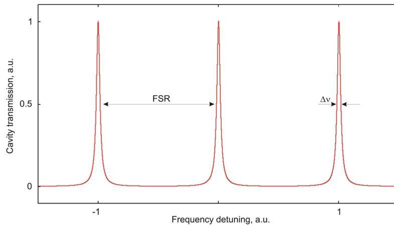
Fig. 2.3.1. Transmission of the cavity
