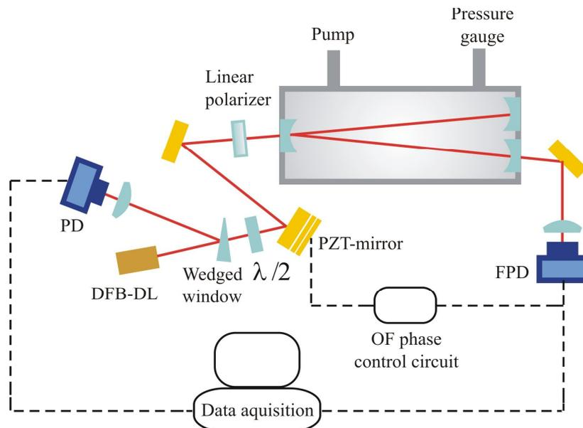
Fig. 2.5.1.2. Sketch of the radiation source of the spectrometer. DFB-DL distributed-feedback diode laser, PD - photodetector, FPD - fast photodetector,  $\lambda/2$  - half wave plate.
