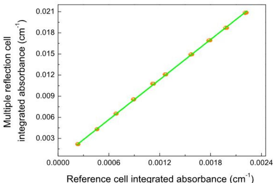
Fig. 4.3.3. Plot of the integrated absorbance in the multiple reflection cell as a function of the same quantity in the reference cell. The slope of the best-fit line is equal to the ratio between the multipass and reference cell lengths.
