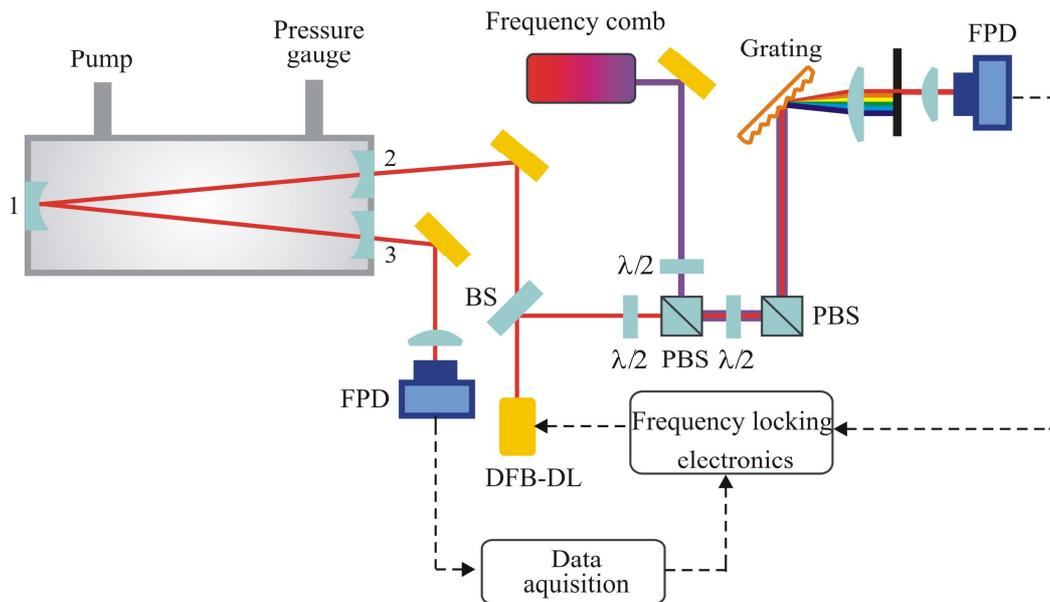
Fig. 3.2.3.1. Sketch of the setup for cavity FSR measurements. DFB-DL distributed-feedback diode laser, FPD - fast photodetector, BS - beam splitter, PBS - polarizing beam splitter,  $\lambda/2$  - half wave plate.
