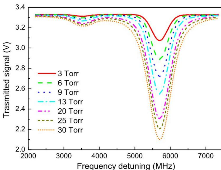
Fig. 4.3.1. Examples of absorption spectra of the  $P_e(14)$  transition of  $C_2H_2$  acquired as a function of the gas pressure. On the horizontal axis the frequency offset of the probe laser with respect to the reference one is reported.
