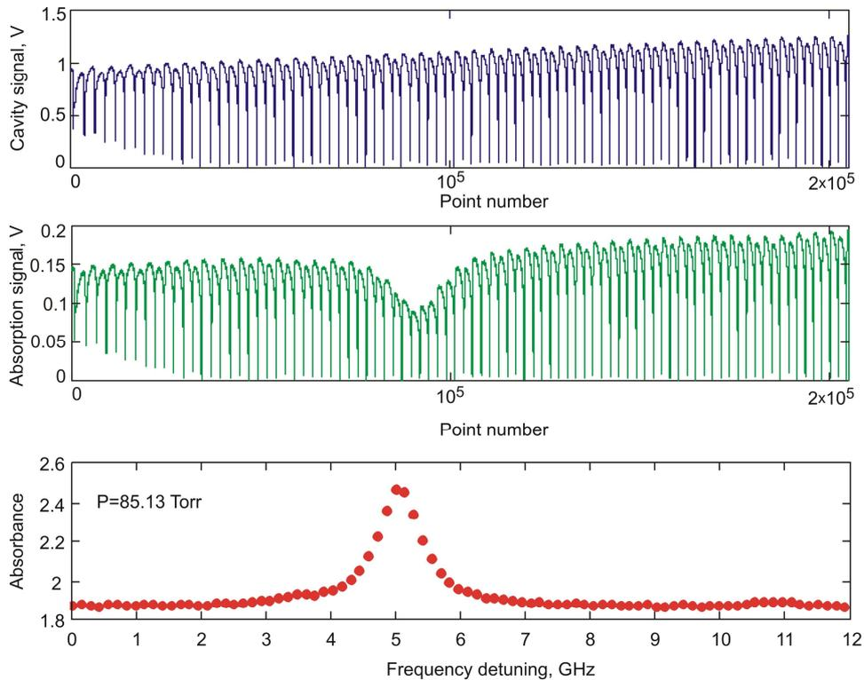
Fig.3.2.1.2. Transmission signal of the V-cavity (1), the signal coming from absorption cell (2), retrieved CO<sub>2</sub> absorption spectrum (3).
