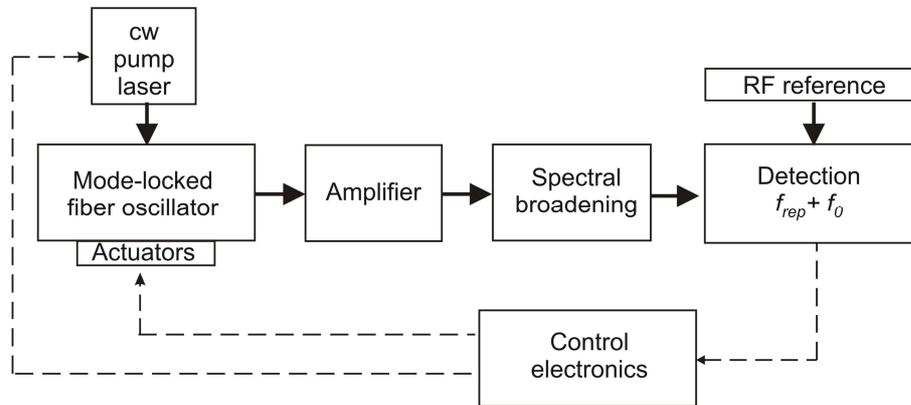
Fig. 2.4.1. Simplified diagram of a typical fiber laser-based frequency comb system. The pulsed output of a fiber laser oscillator is amplified and spectrally broadened. These pulses are then launched into highly nonlinear fiber in which nonlinear processes such as self-phase modulation, self-steepening, four-wave mixing, and Raman scattering spectrally broaden the pulses up to about full octave. The detected signals are used in a control loop for stabilization.
