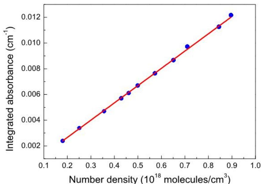
Fig. 4.3.4. Plot of the molecular number density versus the integrated absorbance. The best-fit line exhibits an excellent agreement with the experimental points. The slope of the line provides the quantity  $SL$ . The dispersion of the points, for each pressure, is not visible, being much smaller than the size of the points.
