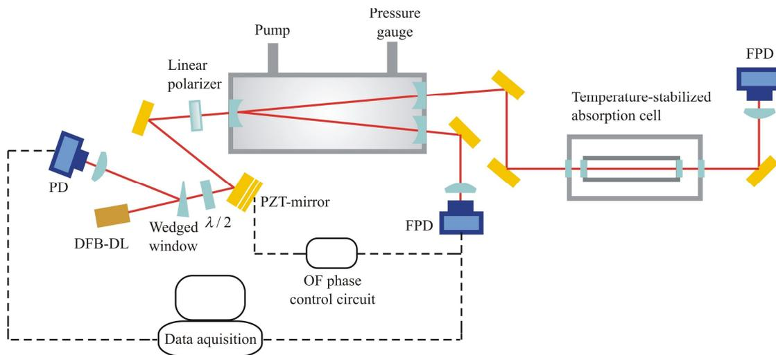
Fig.3.2.1.1. Sketch of the spectrometer. DFB-DL distributed-feedback diode laser, PD - photodetector, FPD - fast photodetector,  $\lambda/2$  - half wave plate.
