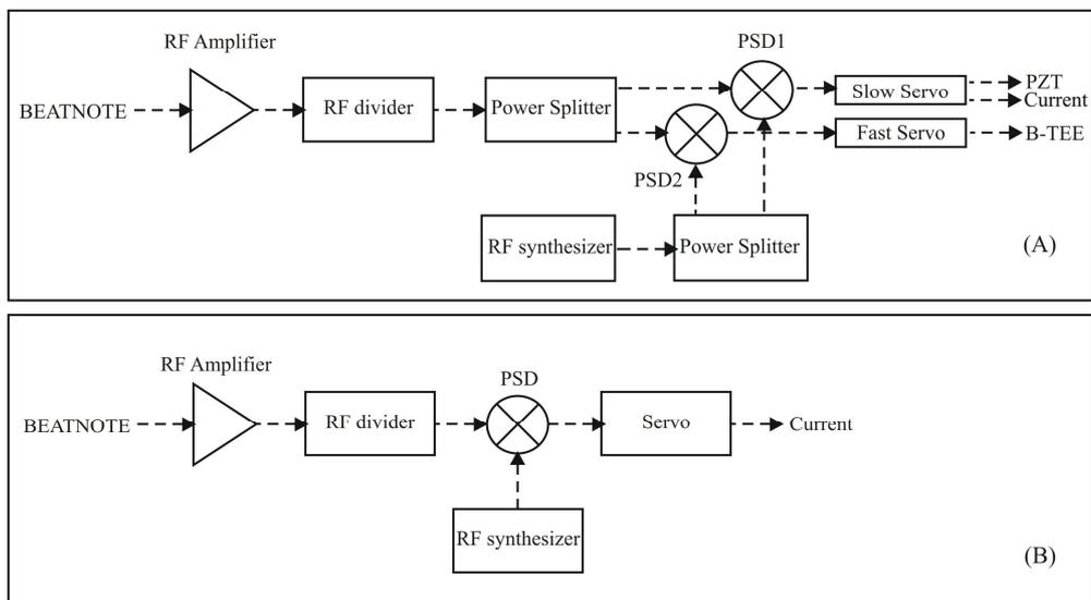
Fig. 2.5.2.1. Scheme of (A) Optical phase-locking loop (OPLL); (B) offset frequency locking (OFL).
