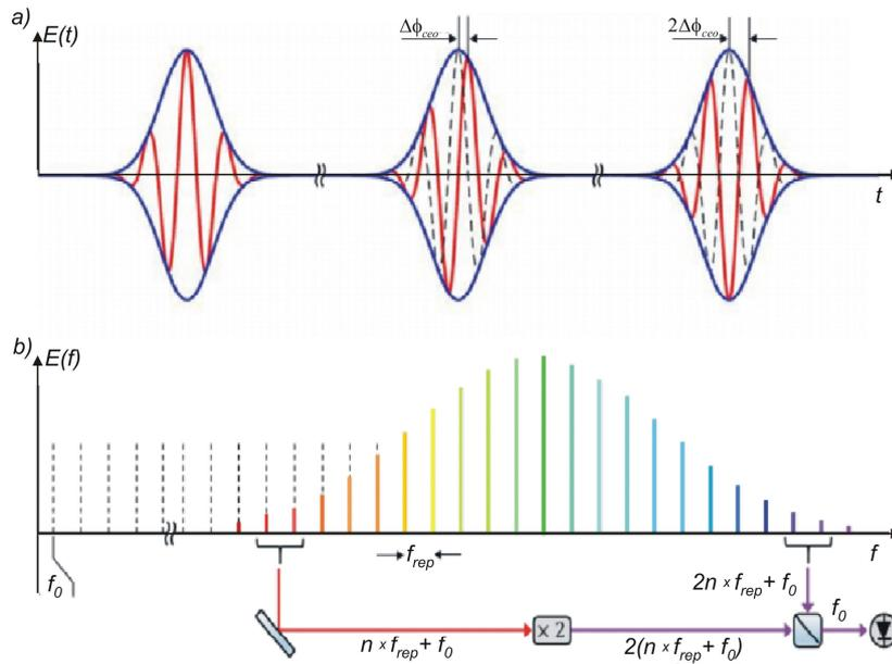
Fig. 2.4.2. Optical pulse train and spectrum emitted by a mode-locked laser. a) The carrier wave (red) and the pulse envelope (blue) travel with different phase and group velocities, leading to a carrier-envelope phase shift. b) The optical spectrum of a mode-locked laser consists of frequency teeth separated by the repetition rate of the laser. The standard method of detecting  $f_{ceo}$  with  $f$ - $2f$  interferometer is shown.
