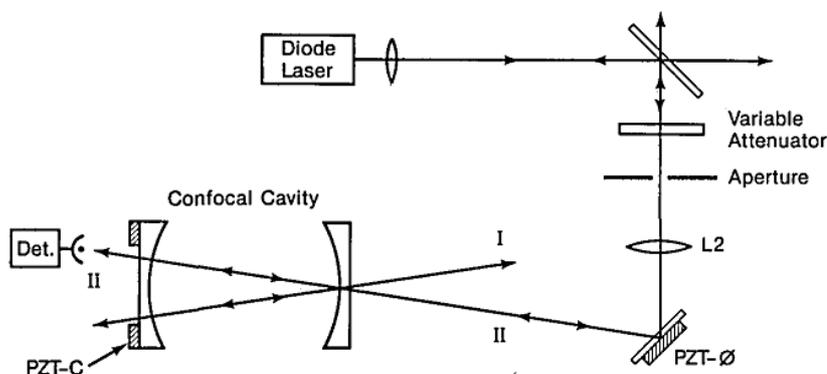
Fig. 2.5.1.1. Schematic the optical feedback locking system [54].
