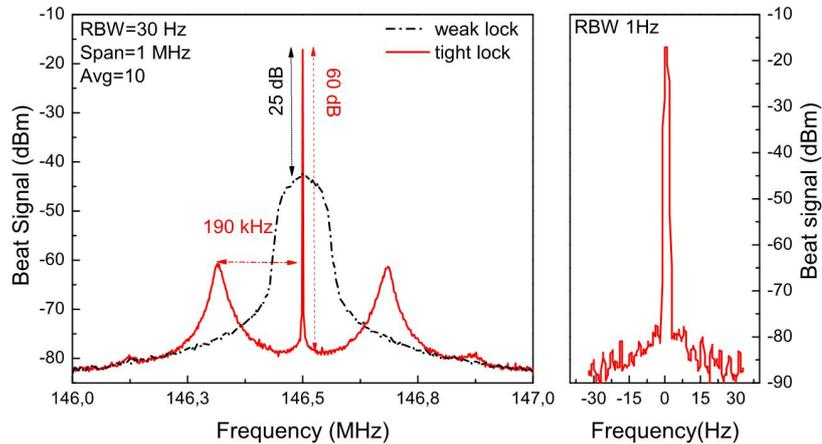
Fig. 2.5.2.2. (a) Example of a beat note between probe and reference lasers under weak (PSD2 deactivated) and tight lock (PSD2 activated) conditions. (b) Beat note under tight lock with higher resolution, characterized by a signal-to-noise ratio of 60 dB, which represents an improvement of 35 dB with respect to the weak lock.
