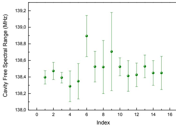
Fig. 3.2.3.2. Determination of the cavity  $FSR$  splitting frequency. Error bar correspond to one standard deviation of 10 values.
