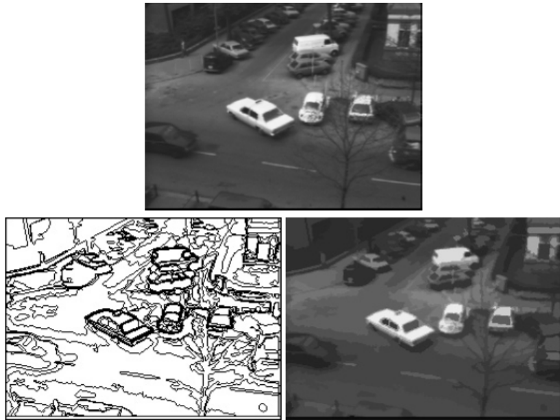
Figure 14: Segmentation result of the Hamburg taxi image obtained minimizing E_{MS}^\lambda with \lambda = 50 using the hierarchy-based algorithm. a) Top: Original image. b) Bottom left: Segmentation boundaries. c) Bottom right: the image \tilde{u} .
