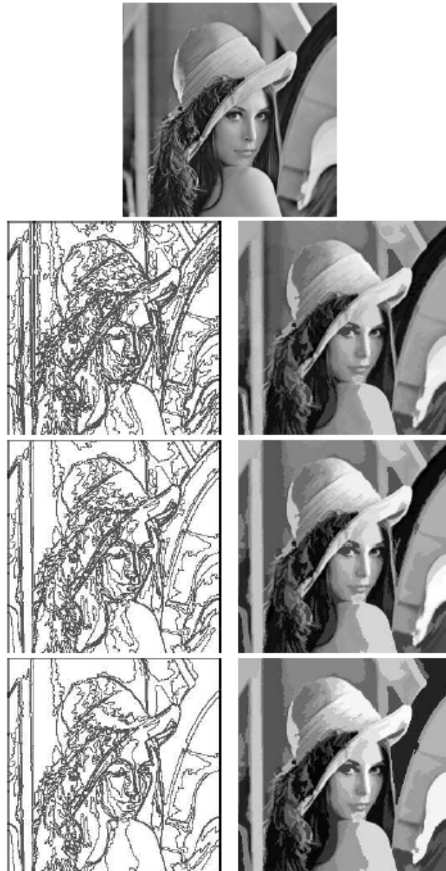
Figure 10: Segmentation result of the Lena image obtained minimizing E_{MS}^{\lambda} with several values of \lambda using the hierarchy-based algorithm. a) First row: original image. Column at the left: segmentation boundaries. Column at the right: image \tilde{u} . b) Second row: \lambda = 20 , c) Third row: \lambda = 60 , d) Forth row: \lambda = 100 .
