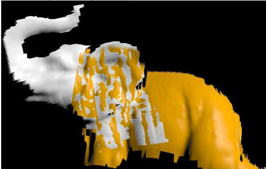
**Figure 2.7: High-speed ICP algorithm applied to scanned data**
