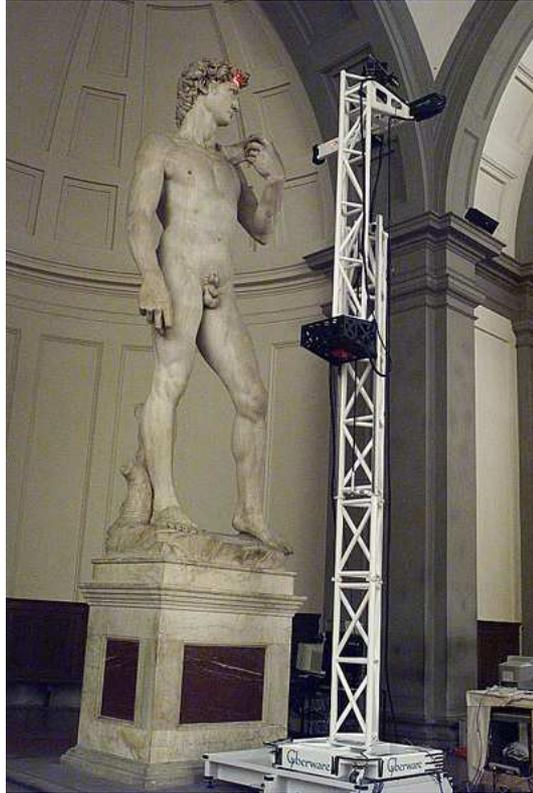
**Figure. 1.8 : Tower 3D laser scanner**
