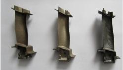
Figure.2: AM manufacturing Inconel 718 turbine blade
