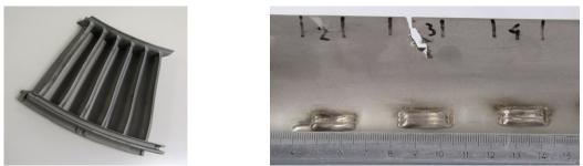
Figure.3: nozzle guide vane repaired with DMD of powder
