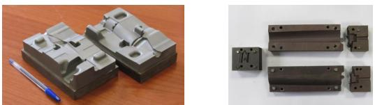
Figure.1: AM-made investment casting moulds for turbine blade
