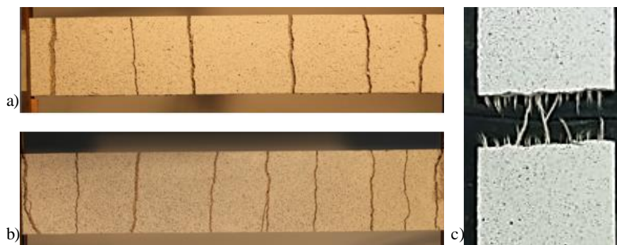
Figure 4.11: a) failure mode of specimens Flax TRM-1L-T-4 and b) Flax TRM-2L-T-4, c) close-up of fabric threads rupture.
