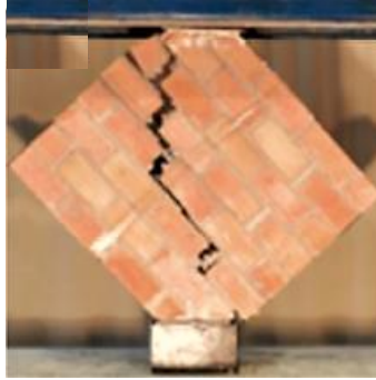
Figure 2.10: Clay brick wall subjected to diagonal compression test [8].
