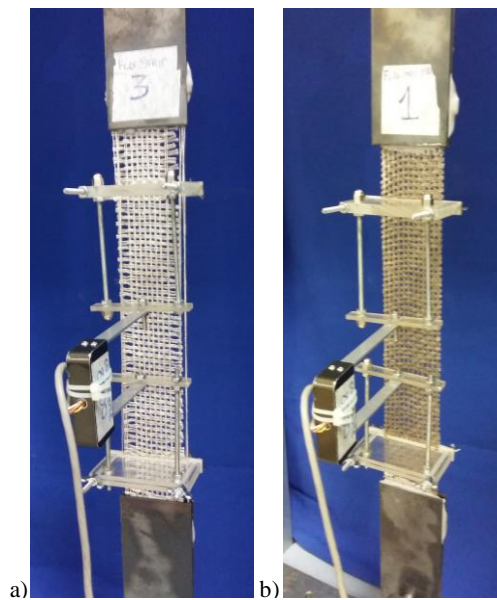
Figure 7.14: Tensile test set up of representative a) Flax fabric 6cm and b) Flax fabric 6cm-imp specimens.
