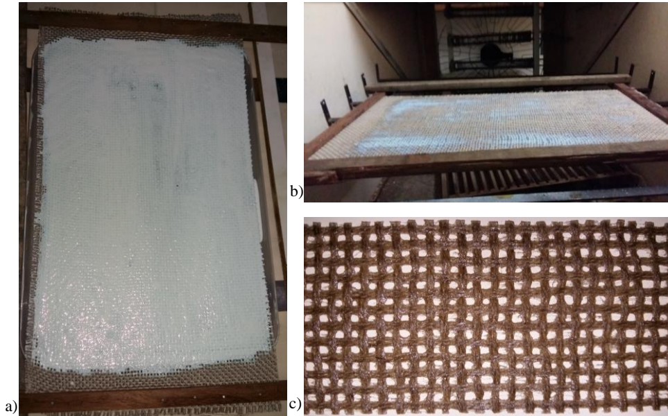
Figure 7.13: Textile impregnation procedure: a) application of the coating substance; b) drying of the textile; c) coated flax strip.
