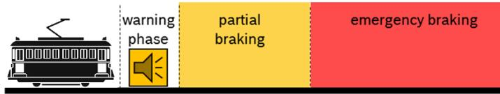
**Figure III.7** Automatic emergency braking protocol for trams
