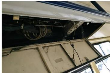
**Figure IV.14** Connection to the RS485 data line in the valance.
