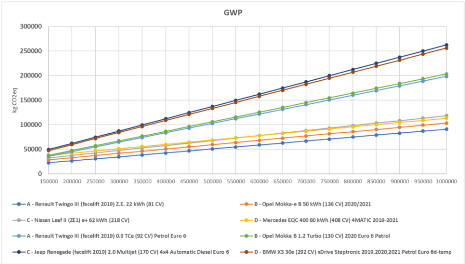
Figure 9: Global warming potential (expressed as kgCO 2 eq vs travelled kilometers) trend for electric and thermal vehicles.
