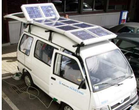
Figure 37 – Micro-Vett porter van, the HSV prototype developed at University of Salerno
