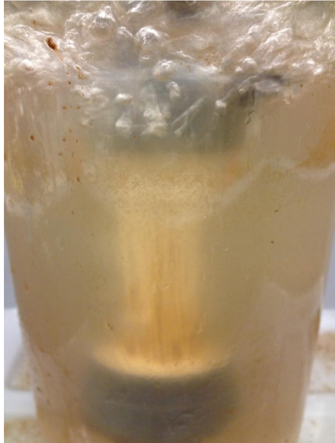
Figure 3-16 - ZW-1 UF membrane installed and fed with biological effluent; air scouring is in place
