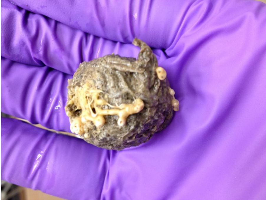
Figure 3-15 - A 2.5 cm diameter bio-ball ready for being fed with wastewater
