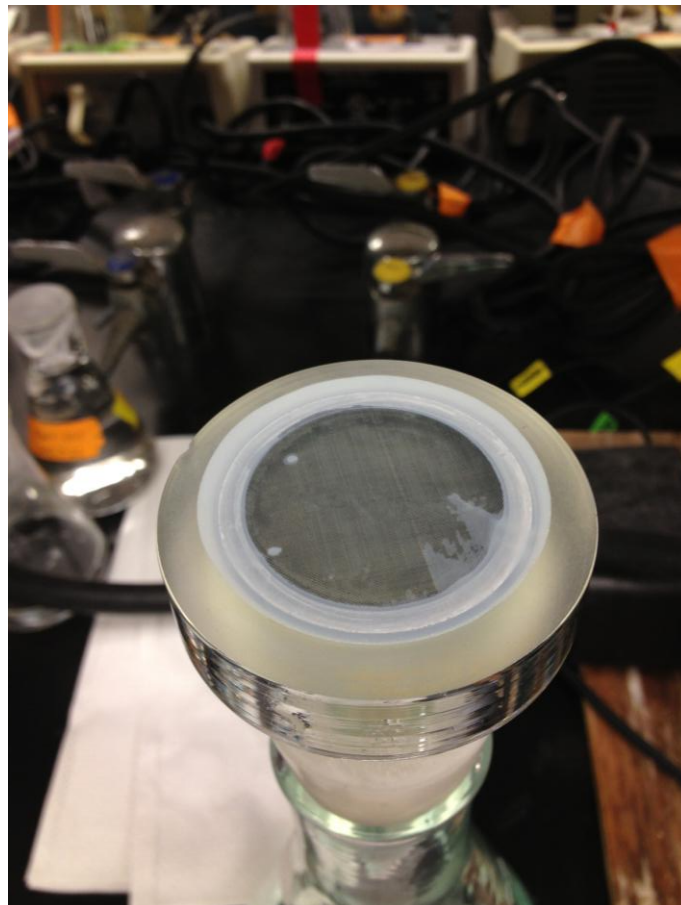
Figure 3-18 - Filtration of samples on a 0.05 \mu\text{m} polycarbonate membrane, and subsequent staining with Alcian Blue
