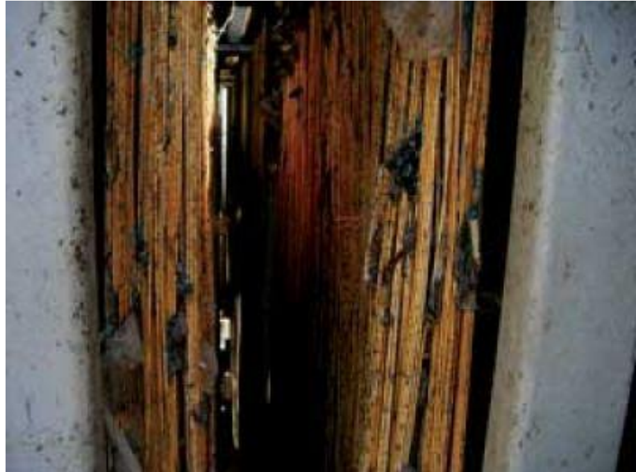
Figure 2-4 - Typical sludging of an hollow fiber MBR
