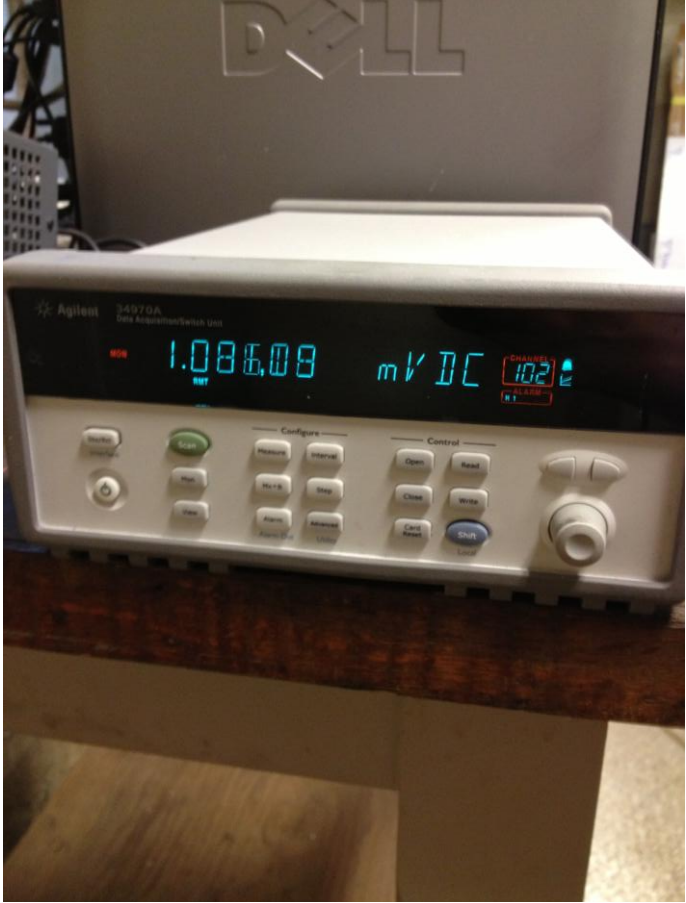
Figure 3-6 - Agilent 34972A data logger (Agilent Instruments, US)
