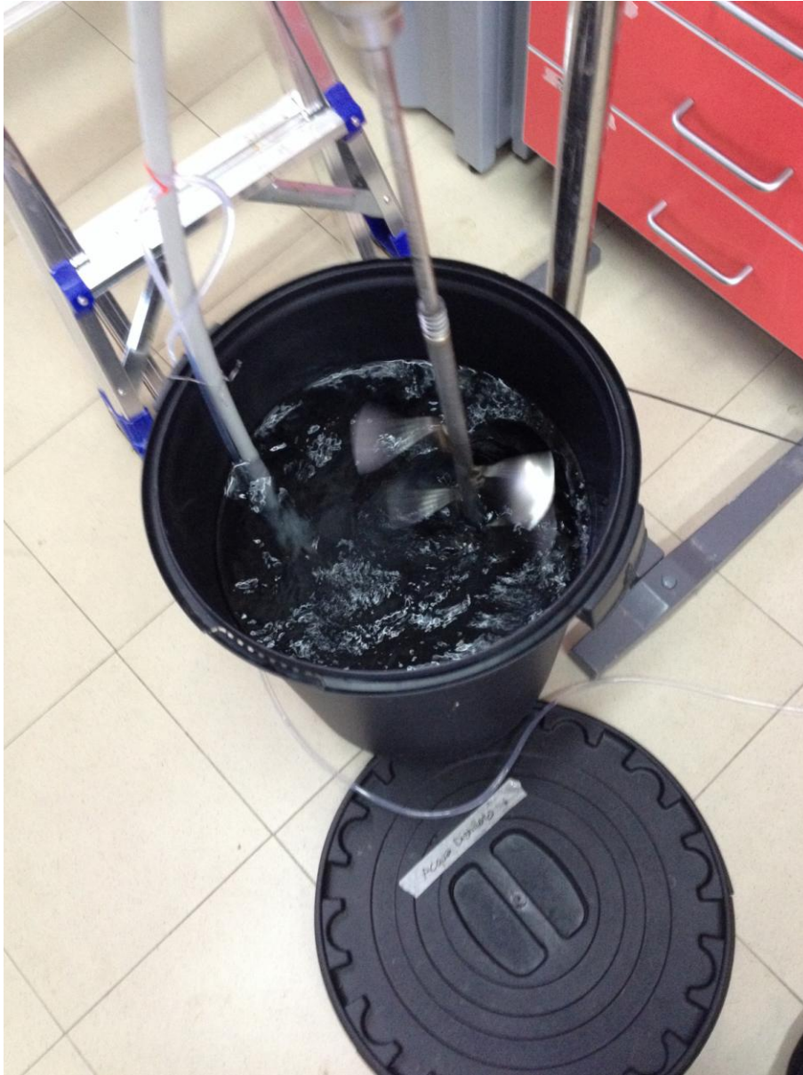
Figure 3-9 - Feedtank (50 L) continuously stirred
