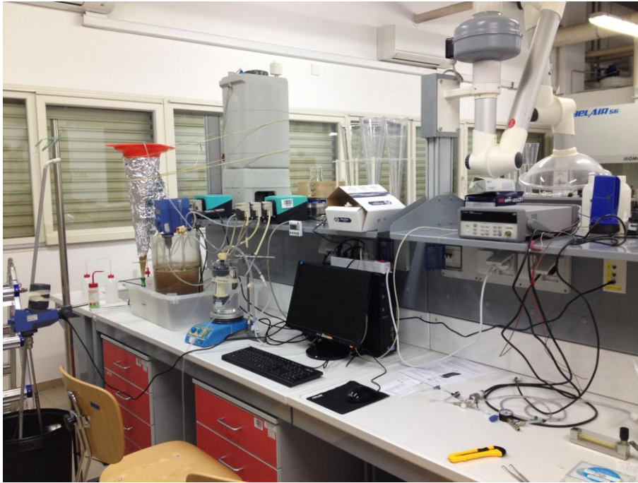
Figure 3-13 - P3 experimental setup, composed of a datalogger, a PC, two peristaltic pumps, a UF membrane, a bioreactor and a temporary settler
