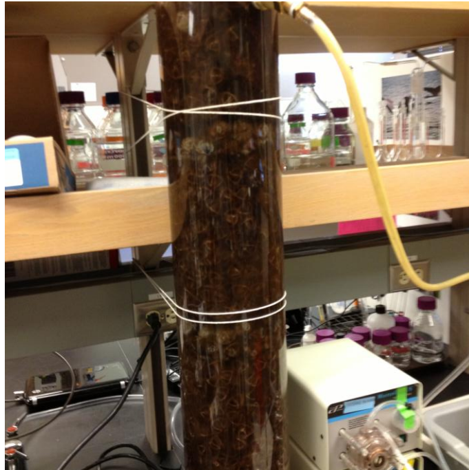
Figure 3-14 - BEMR bioreactor after 3 weeks of operation: biofilm growth can be observed on the internal surface of the reactor
