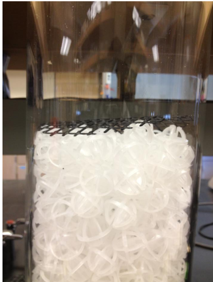
Figure 3-20 - Preparation of the bioreactor with empty plastic carriers to support bio-ball layers
