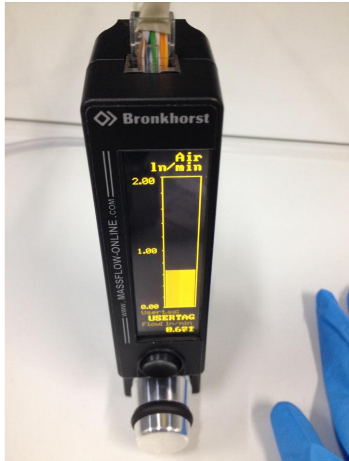
Figure 3-12 - Air flowmeter connected to the datalogger for recording airflow on both biological and membrane steps (Bronkhorst, US)
