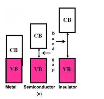
**Figure 1** VB and CB positions in metals, semiconductors, and insulators (Lazar et al., 2012).
