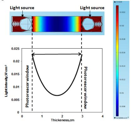
**Figure 121** The Helmholtz model of light distribution inside the reactor; Light sources: UV-lamps with intensity equal to 0.023 W cm<sup>-2</sup>; Reactor thickness: 2.5 cm
