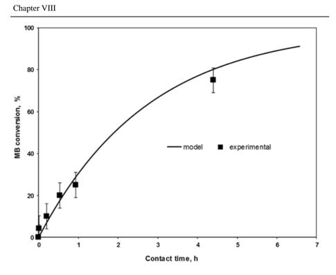
**Figure 126** *Experimental and predict data at different contact times Light sources: UV-lamps; inlet MB concentration. 10ppm*
