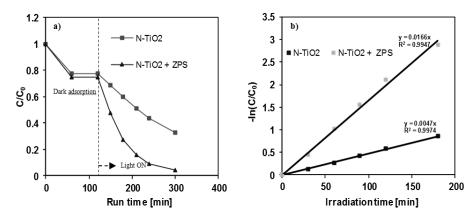
**Figure 95** (a) Decolourization of MB. (b)Evaluation of decolourization kinetic
