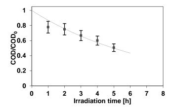
**Figure 67** Comparison between model calculation and experimental data with a catalyst dosage of 3 g/L; catalyst: N-TiO<sub>2</sub>; configuration B; light source: BL strip.
