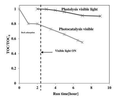
**Figure 42** Comparison between photolysis and photocatalysis (N-TiO<sub>2</sub> dosage : 3g/L) using visible light ( blue LEDs )sources
