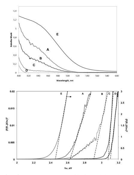
**Figure 87** UV-VIS DRS spectra (a) and band gap calculation (b) for A)  $50N-TiO_2/ZSP$ , B)  $30N-TiO_2/ZSP$ , C)  $15N-TiO_2/ZSP$ , D) ZSP and E)  $N-TiO_2$  photocatalyst.
