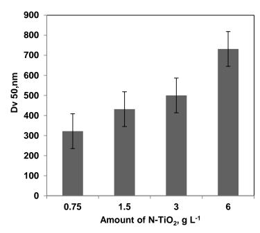
**Figure 71** Effect of amount of N-TiO<sub>2</sub> (0.75-6 g  $L^{-1}$ ) on the Dv 50 size of N-TiO<sub>2</sub> suspensions in bidistilled water solution with AZ concentration of 10 mg  $L^{-1}$ .
