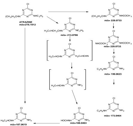
**Figure 103** Possible degradation pathway of atrazine by ZSP under UVA irradiation
