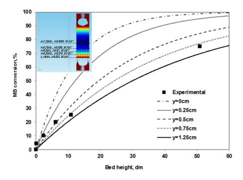
**Figure 127** *MB* conversion as a function of the packed- bed height (*z*-direction) for different distances from the irradiated window (*y*-direction).
