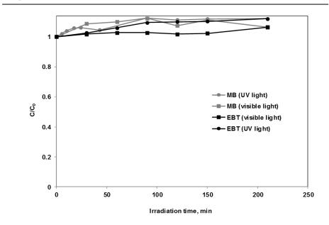
**Figure 113** *Photolysis of MB and EBT in presence of uncoated glass spheres under UV and visible light irradiation*
