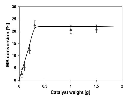
**Figure 33** Evaluation of decolorization after 30 minute with different amount of N\_4 catalyst.
