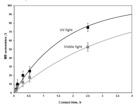
**Figure 123** *MB* conversion profiles as function of contact time using UV or visible light irradiation
