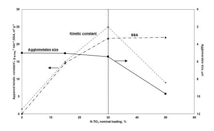
**Figure 100** Atrazine apparent kinetic constant and catalysts agglomerates size as a function of N-TiO<sub>2</sub> nominal loading
