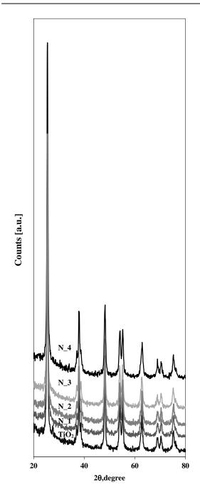
Figure 23 XRD spectra of undoped TiO2, N\_1; N \_2; N \_3; N \_4
