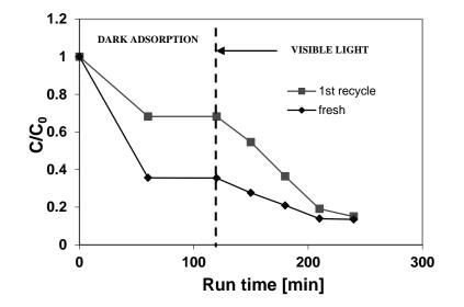
**Figure 36** Evaluation of decolorization performances obtained on  $N_4$  photocatalyst after one recycling experiment. Initial MB concentration 7.5ppm.
