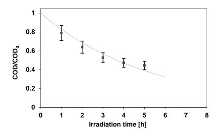
**Figure 63** Comparison between model calculation and experimental data to evaluate the model constant; catalyst: N-TiO<sub>2</sub>; configuration B; catalyst dosage: 3g/L; light source: WL strip
