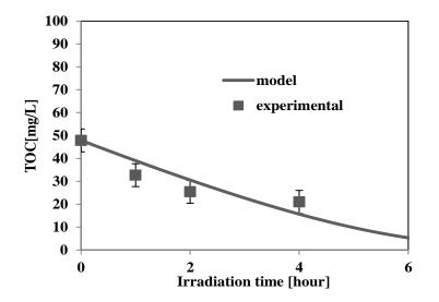
**Figure 55** *Comparison between model calculation and experimental data to find the reaction constant*
