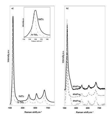
**Figure 110** a) Raman spectra of N-TiO<sub>2</sub> and NdTc samples in the range 100-800 cm<sup>-1</sup> and Raman shift of  $E_g$  modes in the range 110-200 cm<sup>-1</sup>
