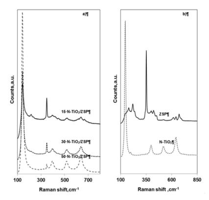
**Figure 89** *a)* Raman spectra of 15 N-TiO<sub>2</sub>/ZSP; 30 N-TiO<sub>2</sub>/ZSP; 50 N-TiO<sub>2</sub>/ZSP samples; b) Raman spectra of ZSP and N-TiO<sub>2</sub> samples
