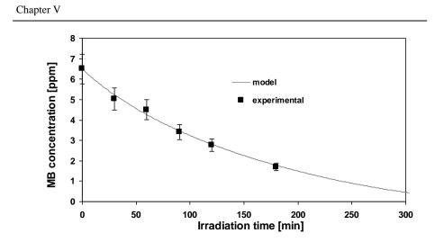
**Figure 51** *Comparison between model calculation and experimental data to find the model constant. Catalyst weight:* 0.3g; *light intensity: 32 mW cm*<sup>-2</sup>.
