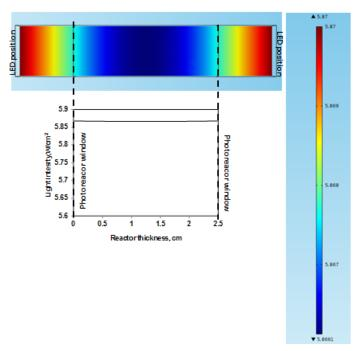
**Figure 128** The Helmholtz model of light distribution inside the reactor; Light sources: UV-LEDs with intensity equal to 5.87 W cm<sup>-2</sup>; Reactor thickness: 2.5cm
