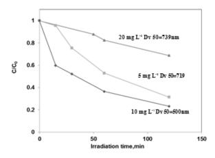
**Figure 76** Photocatalytic decolourization of MB using  $3g L^{-1}$  of N-TiO<sub>2</sub> with different AZ concentration
