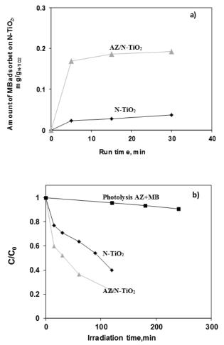
**Figure 75** *a)* Dark adsorption of MB on  $3 \text{ g } L^{-1}$  of N-TiO<sub>2</sub> with and without AZ; b) Photocatalytic decolourization of MB using  $3 \text{ g } L^{-1}$  of N-TiO<sub>2</sub> with and without AZ and photolysis of MB in presence of AZ.
