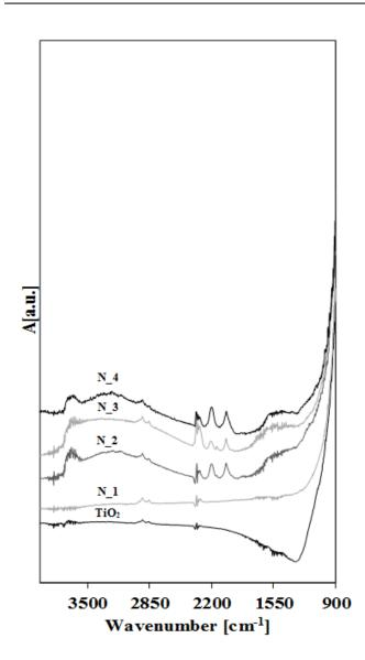
**Figure 22** *FTIR spectra of undoped TiO*<sub>2</sub>, *N*\_1; *N*\_2; *N*\_3; *N*\_4
