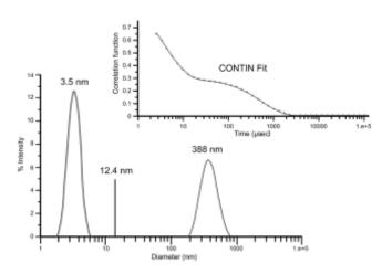
**Figure 18** Correlation curve and CONTIN distribution for 10-mg/mL lysozyme in 100 mMNaCl at 69 °C, measured with a Zetasizer Nano ZS static, dynamic, and electrophoretic light scattering system. The Z average of 12.4 nm is indicated by the solid line in the distribution results.
