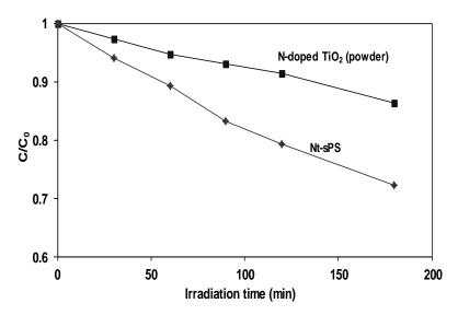
**Figure 83** Comparison of photocatalytic activity of structured photocatalyst (Nt-sPS) with respect to powdered catalyst
