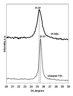
**Figure 108** *XRD patters of NDc of undoped TiO*<sub>2</sub> *and -20 NDc sample in the range 20-30 degree*
