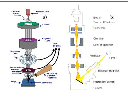
Figure 9 General scheme of a) SEM and b) TEM instrumentations.
