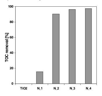
**Figure 31** TOC removal after 180 min of irradiation time ; catalyst weight: 0.3g; initial MB concentration: 7.5 ppm
