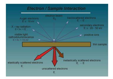
**Figure 8** *Signals generated when a high-energy beam of electrons interacts with a thin specimen.*
