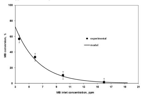
*Figure 125 MB* conversion as a function of inlet concentration; comparison between model calculation and experimental data to find the model constant. Light sources: UV-lamps; liquid flow rate:  $1.451 \text{ h}^{-1}$
