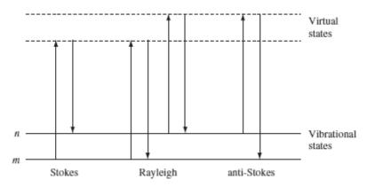
**Figure 12** Diagram of the Rayleigh and Raman scattering processes. The lowest energy vibrational state m is shown at the foot with states of increasing energy above it. Both the low energy (upward arrows) and the scattered energy (downward arrows) have much larger energies than the energy of a vibration.
