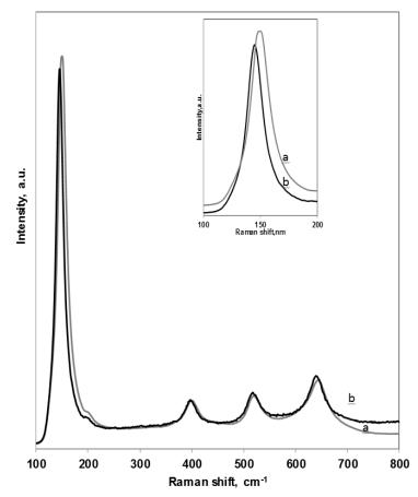
**Figure 106** Raman spectra of (a) 0NDc synthetized by sol-gel method using surface-active agent (Triton X-100) at 0°C and (b) -20NDc synthetized by sol-gel method using surface-active agent (Triton X-100) at -20°C; Raman shift of  $E_g$  modes in the range 100-200cm<sup>-1</sup>(inset)
