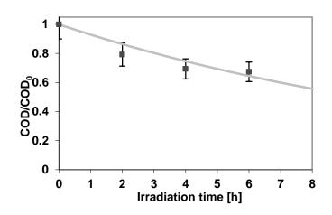
**Figure 65** Comparison between model calculation and experimental data with a catalyst dosage of 3 g/L; catalyst: N-TiO<sub>2</sub>; configuration A; light source: BL
