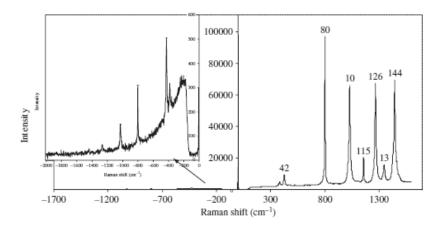
**Figure 13** Stokes and anti-Stokes scattering for cyclohexane. To show the weak anti- Stokes spectrum, the y-axis has been extended in the inset.
