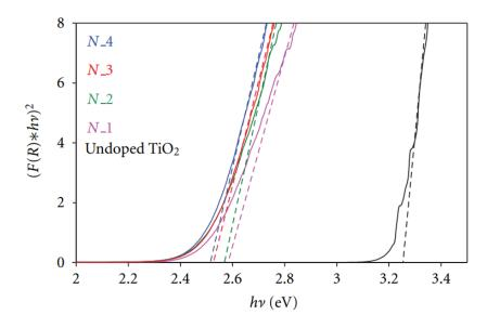
Figure 20 Band-gap estimation from UV-Vis DRS.
