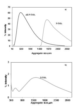
**Figure 69** *a*) Aggregate size distribution of N-TiO<sub>2</sub> with and without azulene in range 10-3000 nm; b) Aggregate size distribution of N-TiO<sub>2</sub> without azulene in range 300-3000  $\mu$ m
