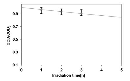
**Figure 68** Comparison between model calculation and experimental data with a catalyst dosage of 3 g/L; catalyst: N-TiO<sub>2</sub>; configuration B; light source: UV lamp.
