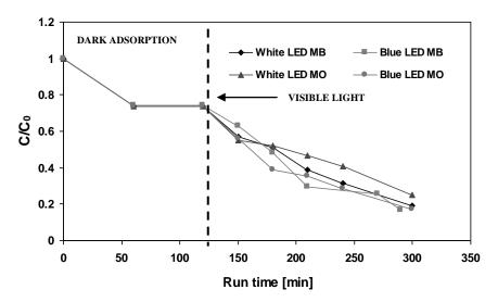
**Figure 35** Evaluation of decolorization with different dyes and different light source; initial MB and MO concentration:9 ppm
