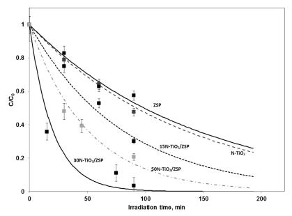
**Figure 99** Behavior of atrazine experimental concentration ( ) and predicted data( - ) as function of irradiation time for the different photocatalysts
