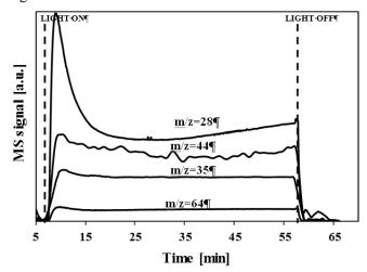
**Figure 49** Outlet reactor concentration (a.u.) of chlorine (m/z) 35, nitrogen (m/z) 28, carbon dioxide (m/z) 44, and sulphur dioxide (m/z) 64, as a function of run time. Initial cyclohexane concentration 10 ppm; incident light intensity  $32mW/cm^2$ .
