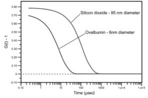
**Figure 17** Intensity correlation curves for ovalbumin and silicon dioxide, measured with a Zetasizer Nano ZS static, dynamic, and electrophoretic light scattering instrument.
