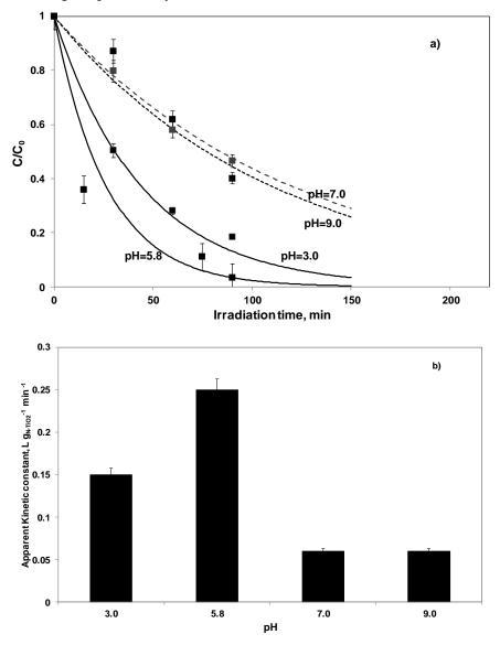
**Figure 102** *a)* Photocatalytic removal of atrazine on  $30N-TiO_2/ZSP$  at different initial pH values, and b) apparent kinetic constant at different initial pH values.
