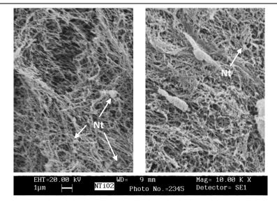
Figure 81 SEM image of Nt-sPS aerogel
