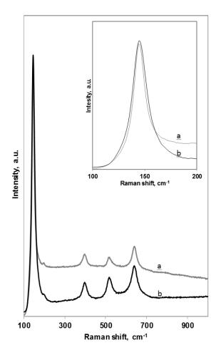
**Figure 105** Raman spectra of (a) N-TiO<sub>2</sub> synthetized by sol-gel method at 0°C and (b) 0NDc synthetized by sol-gel method at 0°C using surface-active agent (Triton X-100); Raman shift of  $E_g$  modes in the range 110-200 cm<sup>-1</sup> (inset)
