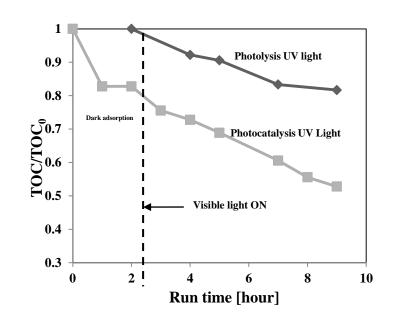
**Figure 40** Comparison between photolysis and photocatalysis (N-TiO<sub>2</sub> dosage: 3g/L) using UV light sources
