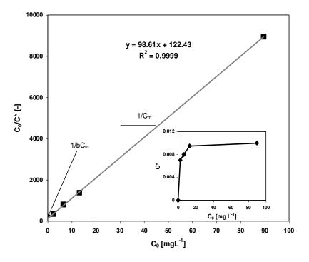
**Figure 50** Evaluation of MB adsorption constant and amount of MB adsorbed on N-doped  $TiO_2$  (inset)
