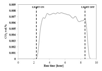
**Figure 41** Gas phase analysis during photocatalysis in presence of UV irradiation.
