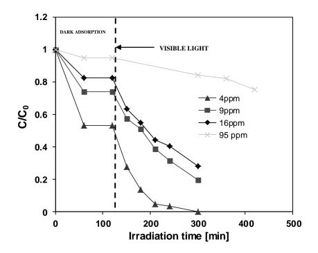
**Figure 34** Evaluation of decolorization with different initial concentration of MB; catalyst: N\_4
