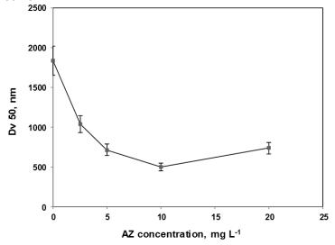
**Figure 70** Effect of concentration of AZ (2.5-20 mg  $L^{-1}$ ) on the Dv 50 size of N-TiO<sub>2</sub> suspensions; N-TiO<sub>2</sub> dosage:  $3g L^{-1}$ .
