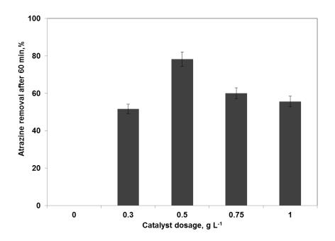
Figure 101 Effect of 30N-TiO<sub>2</sub>/ZSP dosage on the removal of atrazine.
