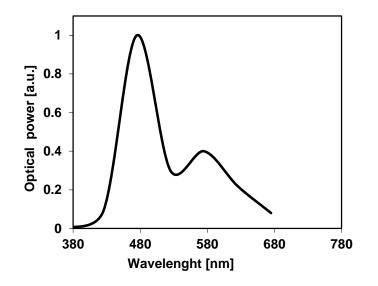
Figure 47 Emission spectrum of the white LEDs
