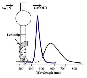
**Figure 28** Emission spectum of the light sources and schematic picture of the photoreactor.
