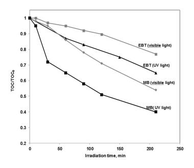
**Figure 117** *Photocatalytic mineralization of MB and EBT under UV and visible light irradiation on 4 NdTcg*
