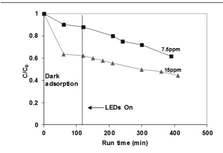
**Figure 84** Evaluation of solution decolourization with different initial *MB* concentration.
