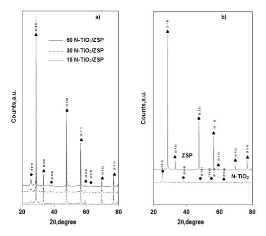
**Figure 88** *a)* XRD patterns of 15 N-TiO<sub>2</sub>/ZSP; 30 N-TiO<sub>2</sub>/ZSP; 50 N-TiO<sub>2</sub>/ZSP samples; b) XRD patterns spectra of ZSP and N-TiO<sub>2</sub> samples. Legend:triangle=ZSP (Sphalerite cubic phase); diamond= N-TiO<sub>2</sub> (anatase)
