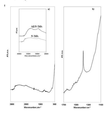
**Figure 72** a) FTIR spectra of N-TiO<sub>2</sub> b) The FTIR difference spectra of AZ/N-TiO<sub>2</sub>
