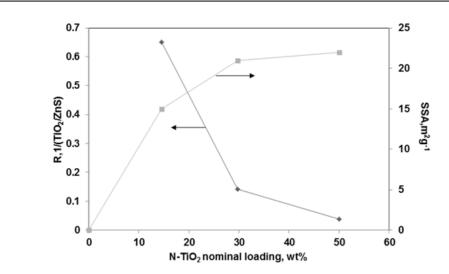
**Figure 90** *Ratio between the maximum intensity of the phosphors* peaks at about 350 cm<sup>-1</sup> and the maximum intensity of titania peak at 144 cm<sup>-1</sup> and SSA (BET) trend function of N-TiO<sub>2</sub> nominal loading
