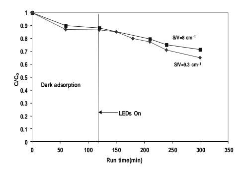
**Figure 85** Influence of different surface-volume ratio (S/V) on photocatalytic activity
