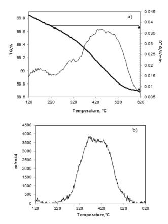
**Figure 74** *a*) *TG* analysis of AZ/N-TiO<sub>2</sub> sample; b) MS result of AZ/N-TiO<sub>2</sub> sample
