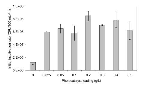
**Figure 44** Initial inactivation rate as a function of N-TiO<sub>2</sub> loading
