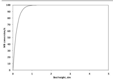
**Figure 129** Simulated MB conversion as function of z-direction, Light sources: UV-LEDs; MB concentration: 10 ppm
