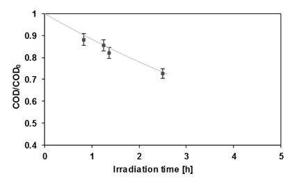
**Figure 64** Comparison between model calculation and experimental data with a catalyst dosage of 1.5g/L; catalyst: N-TiO<sub>2</sub>; configuration B; light source: WL strip.
