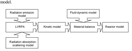
**Figure 5** Schematic representation of the modeling of a photocatalytic reactor
