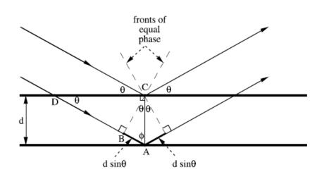
**Figure 7** Geometry for interference of a wave scattered from two planesseparated by a spacing, d. The dashed lines are parallel to the crests or troughs of the incident and diffracted wavefronts. The important path length difference for the two rays is the sum of the two dark segments
