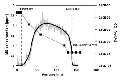
**Figure 48** Decolorization of MB under visible light generated by white LEDs; catalyst weight: 0.3g; initial MB concentration: 7.5ppm and gas analysis of  $CO_2$  during visible irradiation of MB solution
