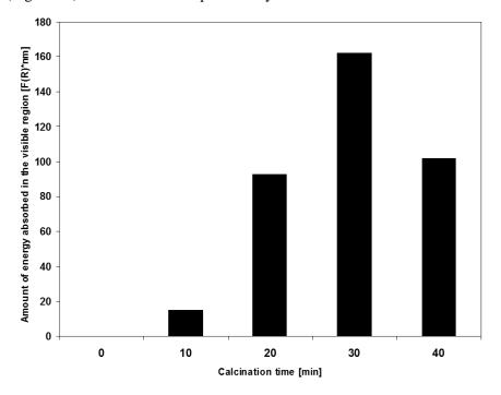
**Figure 24** Amount of energy absorbed in visible region by  $N_4$  catalyst as a function of calcination time.
