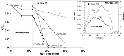
**Figure 97** Comparison of core-shell photocatalysts performances by varying the extent of N-doped  $TiO_2$  shell (indicated by the different weight percentages of N-doped  $TiO_2$ ) in photocatalytic decolourization of MB and gas-phase analysis of 30%NTiO<sub>2</sub>-ZSP
