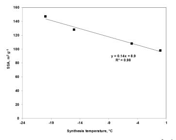
**Figure 109** Trend of NdTc specific surface area  $(m^2 g^{-1})$  as a function of sol-gel synthesis reaction temperature
