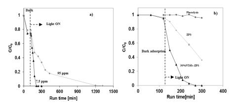
**Figure 98** *a)* Evaluation of decolourization with different initial concentration of MB; photocatalyst: 30%NTiO<sub>2</sub>-ZSP; *b)* Evaluation of MO decolourization); photocatalysts 30%NTiO<sub>2</sub>-ZSP
