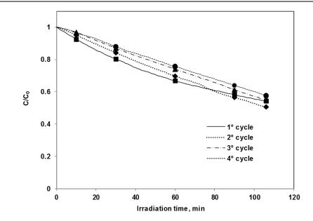
**Figure 115** Evaluation of MB decolourization performances obtained on 4NdTcg after 4 recycling experiments.
