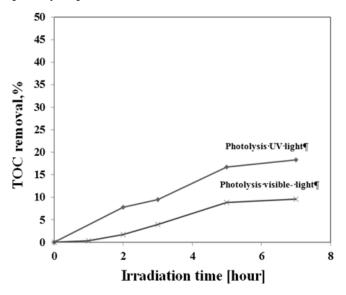
Figure 39 Comparison between photolysis under visible light and UV light
