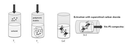
Figure 78 Nt-sPS composites step of synthesis
