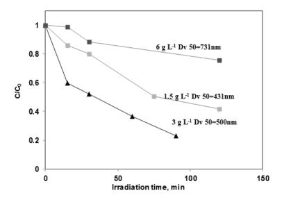
**Figure 77** Photocatalytic decolourization of MB (AZ concentration 10 mg  $L^{-1}$ ) using different amount of N-TiO<sub>2</sub> (1.5 - 6g  $L^{-1}$ )
