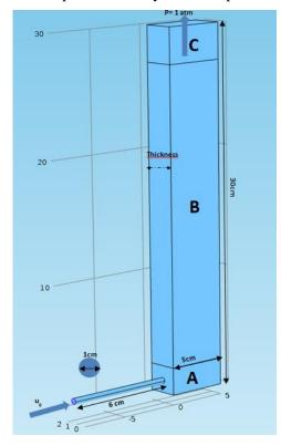
**Figure 118** *Preliminary domain for the fluid dynamic model where a) is the homogenization zone; b) is the body of reactor where is settled the structured photocatalyst bed; c) the outlet zone*
