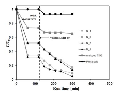
**Figure 29** Decolorization of MB under visible light generated by white LEDs; catalyst weight: 0.3g; initial MB concentration: 7.5 ppm
