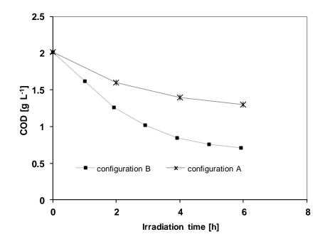
**Figure 59** Comparison between photoreactor configuration A and configuration B using white LEDs and N-TiO<sub>2</sub> catalyst; catalyst dosage: 3g/L
