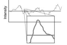
**Figure 16** Intensity time trace showing the lack of discontinuity expected for arandom signal when viewed across a short time interval
