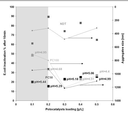
**Figure 45** *E.* coli inactivation ( $\blacksquare$ ) and aggregates size ( $\bigcirc$ ) as a function of photocatalysts loading with pH value of the suspension for each photocatalyst loading
