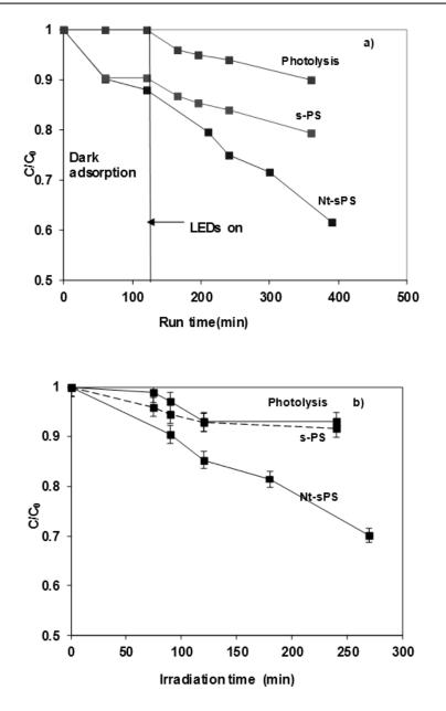
**Figure 82** Comparison between the photocatalytic activity of s-PS aerogel and the photocatalyst dispersed in the polymeric substrate (Nt-sPS) as a function of run time (a) and as a function of irradiation time (b)
