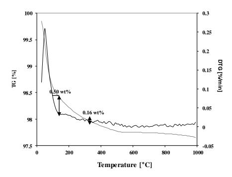
Figure 25 TG analysis of N\_4 photocatalyst
