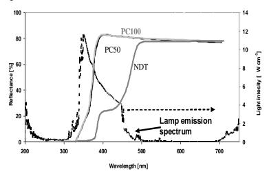
**Figure 43** *Comparison between UV-Vis spectra of PC50, PC100 and NDT photocatalysts and emission spectrum of lamp*
