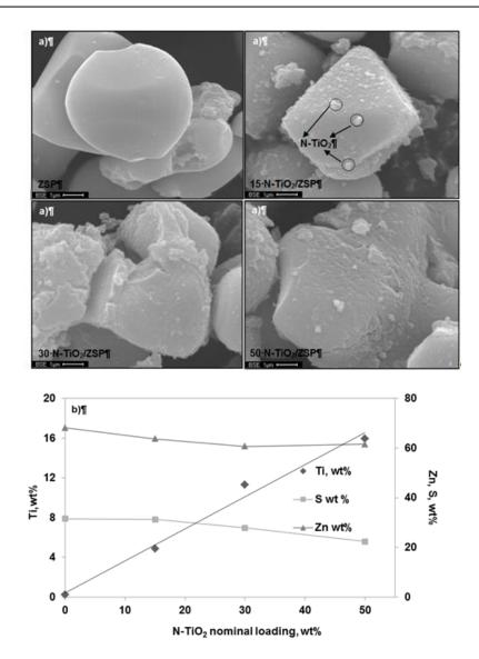
**Figure 91** *a)* SEM images and b)EDAX analysis of the samples ZSP; 15 N-TiO<sub>2</sub>/ZSP; 30 N-TiO<sub>2</sub>/ZSP; 50 N-TiO<sub>2</sub>/ZSP
