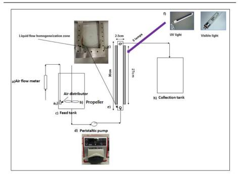
**Figure 122** *Experimental set up apparatus: (a) air flow meter;(a<sub>1</sub>) air distributor; (b) propeller; (c) feed tank; (d) peristaltic pump, (e) inlet of the flow in the reactor; (f) light sources; (g) outlet of liquid flow; (h) collection tank.*
