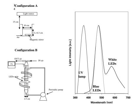
**Figure 57** *Reactor configurations (A and B) and emission spectrum of the different light sources*
