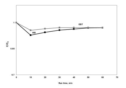
Figure 112 Dark adsorption of MB and EBT on uncoated glass spheres
