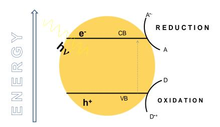
Figure 2 Illustration of the main processes occurring on a semiconductor particle under electronic excitation
