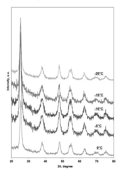
Figure 107 XRD patters of NdTc at different synthesis reaction temperature
