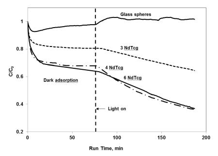
**Figure 114** *Photocatalytic decolourization of MB under UV light irradiation (optimization of NdTc amount on glass sphere)*
