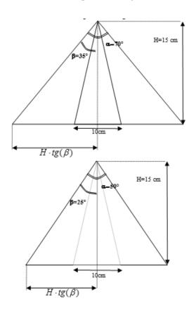
**Figure 61** Geometric schematization of light flux upper the photoreactor (configuration A)
