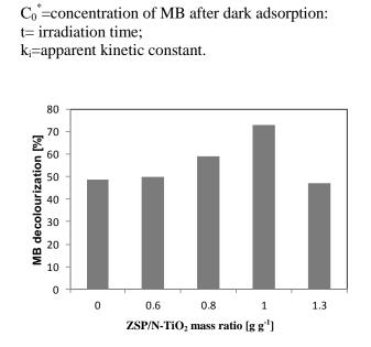
**Figure 96** Evaluation of the effect of different amount of ZPS in physical combination with the similar amount of N-TiO<sub>2</sub> (0.3 g) on the decolourization of MB after one hour
