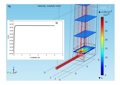
*Figure 120 a) The flow lines along the photoreactor, b) Flat profile inside the packed bed*
