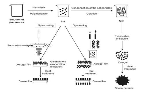
Figure 6 Schematic overview of the sol-gel process (Larry et al. 1990)
