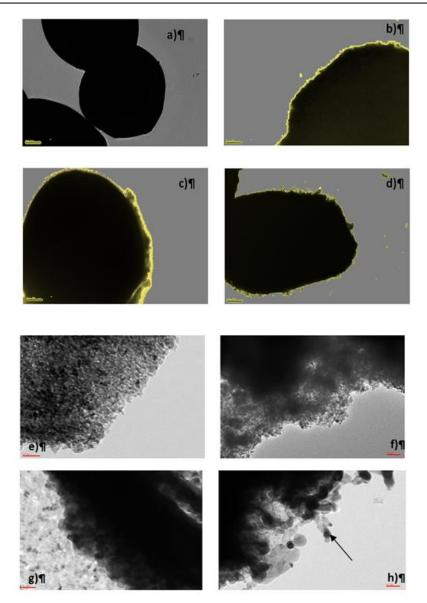
**Figure 92** *TEM images: a)ZSP; b)15 N*-*TiO*<sub>2</sub>/*ZSP; c) 30 N*-*TiO*<sub>2</sub>/*ZSP; d)50 N*-*TiO*<sub>2</sub>/*ZSP (scale bar equals 5 \mum) and e) N*-*TiO*<sub>2</sub>; f)15 *N*-*TiO*<sub>2</sub>/*ZSP; g) 30 N*-*TiO*<sub>2</sub>/*ZSP; h)50 N*-*TiO*<sub>2</sub>/*ZSP (scale bar equals 50 nm).*
