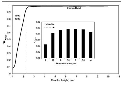
**Figure 119** Behavior of  $\overline{v}/v_{\text{max}}$  as a function of reactor height (z-direction) and behavior of  $\overline{v}/v_{\text{max}}$  as a function of reactor thickness at the bed inlet (inset).
