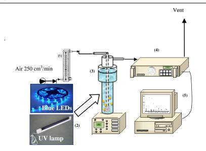
**Figure 38** Experimental set up apparatus (1) flow meter; (2) magnetic stirrer; (3) photoreactor; (4)  $CO_2$  analyzer, (5) personal computer for data acquisition.
