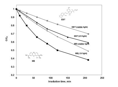
**Figure 116** *Photocatalytic decolourization of MB and EBT under UV and visible light irradiation on 4NdTcg*
