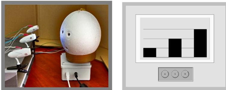
**Figure 4.2.** The first experiment involved turning a robotic head toward lights; the scene was hidden in a box to the user, which had only visual cues on monitors appearing as histograms (stimuli to learn) and buttons (action to select).
