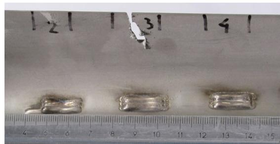
Figure.3: nozzle guide vane repaired with DMD of powder
