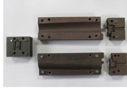
Figure.1: AM-made investment casting moulds for turbine blade
