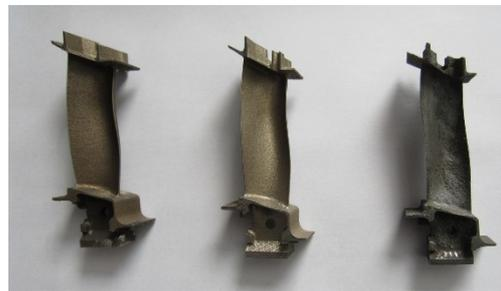
Figure.2: AM manufacturing Inconel 718 turbine blade
