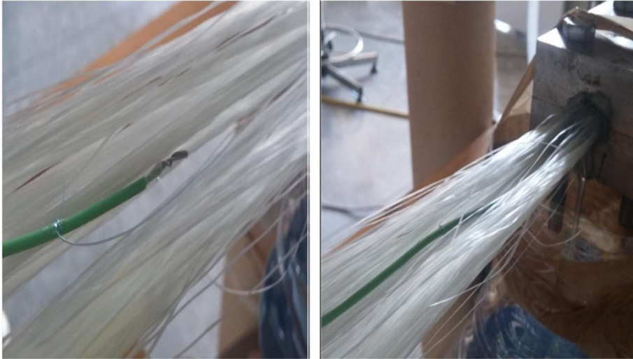
Figure IV.4 Thermocouple fixing on the advancing fibers.
