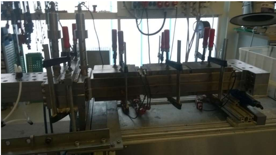
Figure IV.5 Curing-forming injection pultrusion die at Fraunhofer IGCV.
