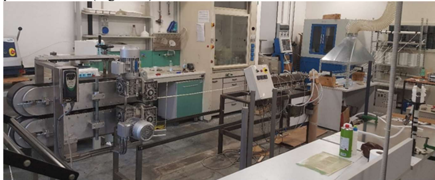
Figure IV.1 Laboratory-scale injection pultrusion line.
