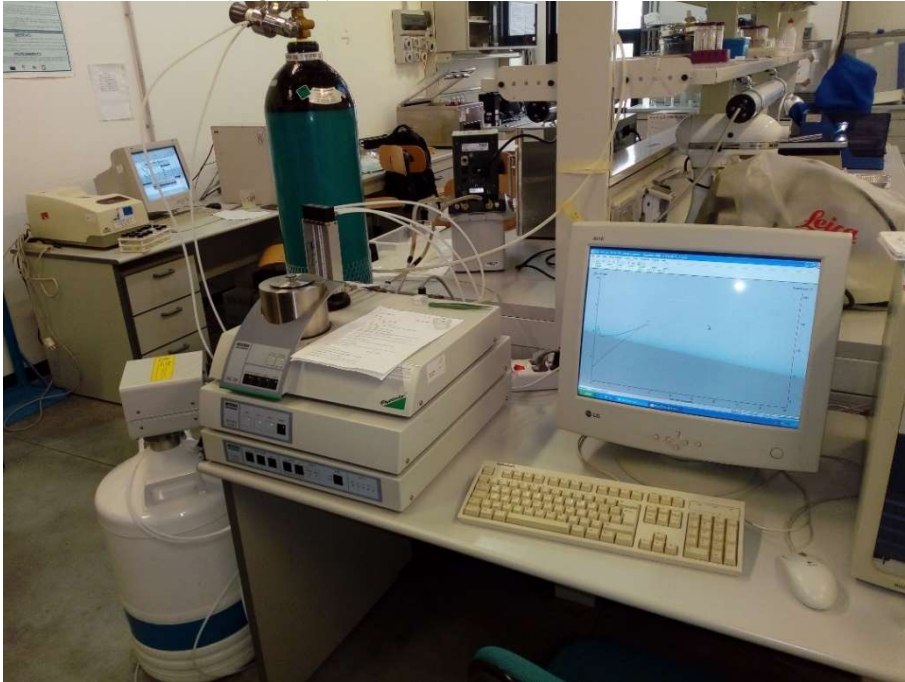
Figure II.2 Differential scanning calorimetry Netzsch DSC 204 equipment.
