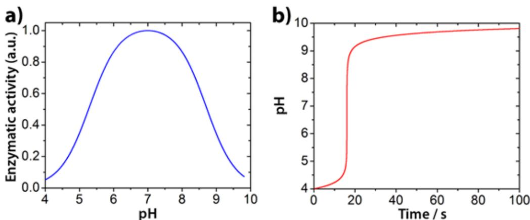
**Figure 1:** The characteristics of the urea-urease reaction. a) Dependence of the urea-urease reaction rate upon the pH in unbuffered solutions. b) autocatalytic profile of the pH during the urea-urease reaction.
