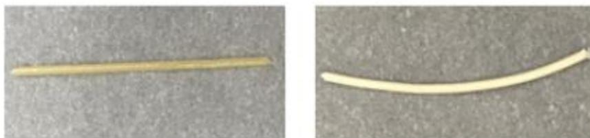
*Figure 14. Filaments obtained via HME with 80% of PVA and 20% of APIs (left: Carvedilod, right: Haloperidol) (developed by Wei et al., 2020)*
