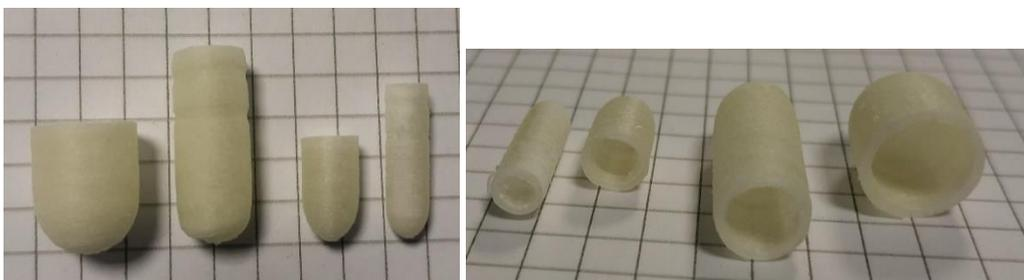
*Figure 2.9. MW drug loaded models in Acetone PEG solution using the best loading cycle with PEG (5 x 10'' 40-80°C at 100W)*
