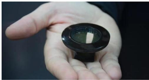
*Figure 7. The first-ever 3D printed part: an eye-wash cup*
