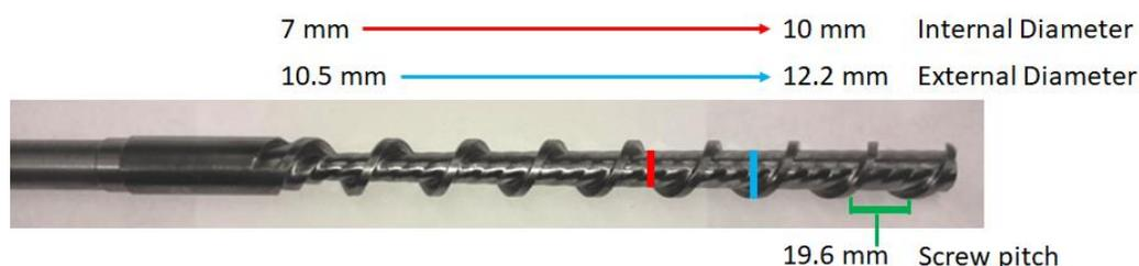
*Fig. 1.1: Screw configuration of the single-screw extruder*
