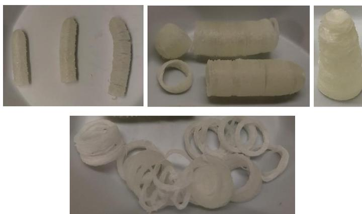
*Figure 2.6. Delamination and/or breakage after MW irradiation of bodies2 processed in:*
