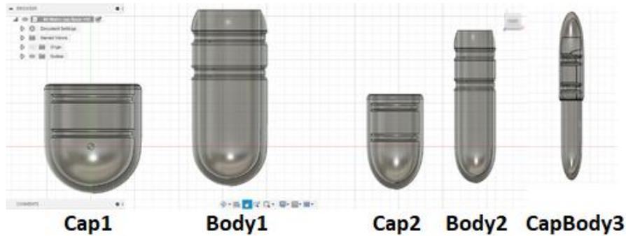
*Figure 2.1: Digital models of the caps and bodies for 3D printing of caps-in-cap systems*
