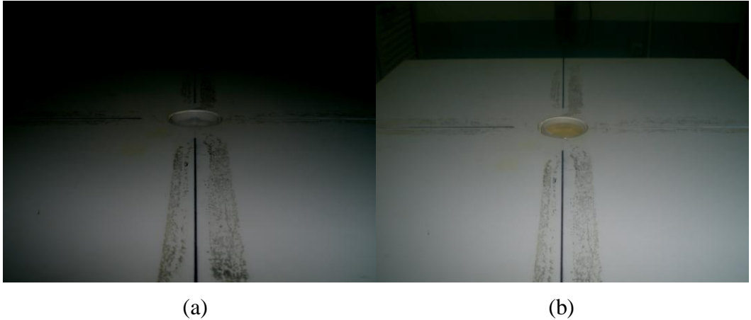
Fig. 2.3 hole containing the sample in the plastic water sheets (a) before and (b) after (21Gy) irradiation.
