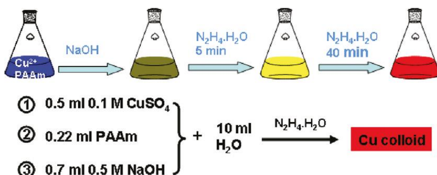
Fig. 3.1: schematic illustration of the procedure used for copper nanoparticles formation [6].
