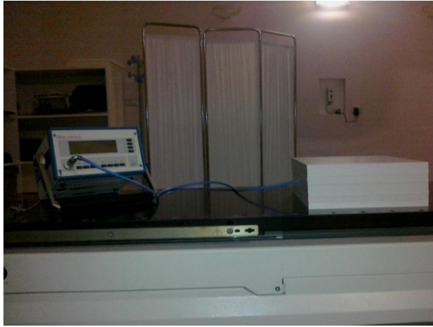
Fig. 1.13: ionization chamber 30013 Farmer, connected to the electrometer PTW UNIDOS.
