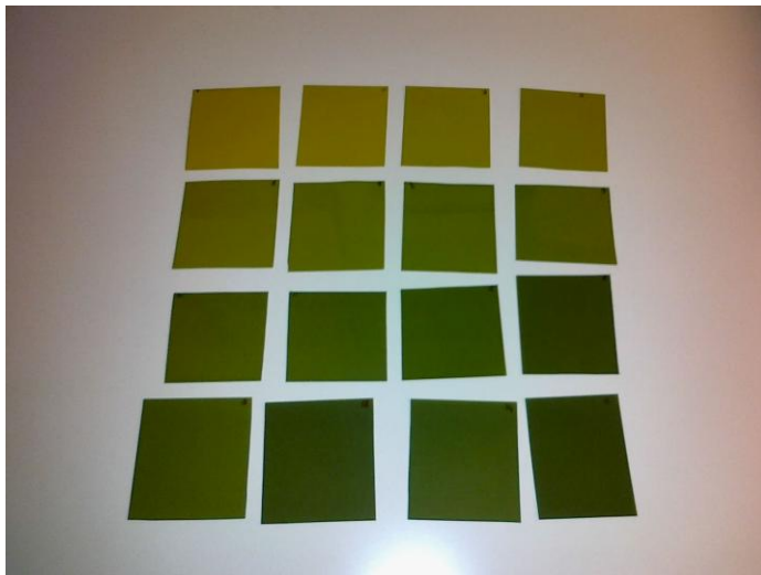
Fig. 1.14: not irradiated sample (up left); the irradiated samples (in total 15) show a different color according to the dose.
