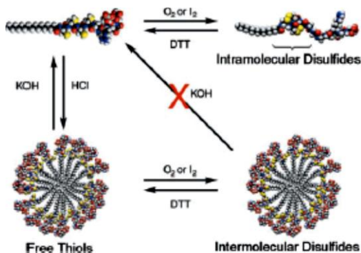
Figure 3.3: Schematic representation of the self-assembly and covalent linkage of the PAs based on pH and oxidation state.
