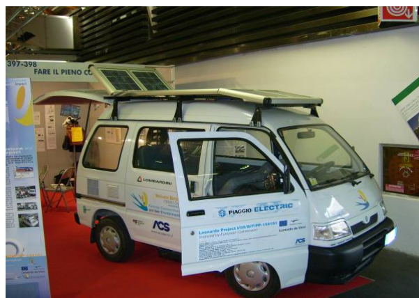
Figure 1.7 – Piaggio Porter solar hybrid vehicle prototype
