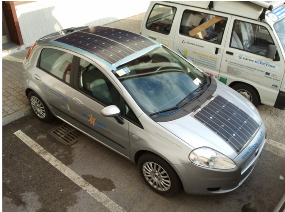
Figure 3.10 – PV panels installed on Fiat Grande Punto
