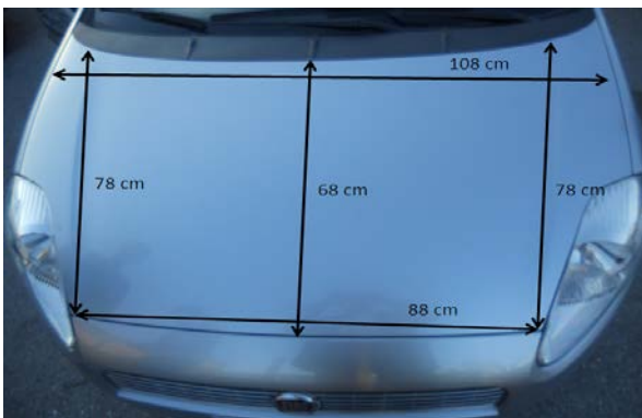
Figure 2.10 - Useful surface on prototype bonnet
