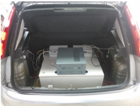
Figure 3.5 – Battery pack, IWM drivers and control system arrangement in vehicle hood
