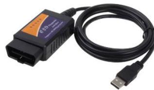
Figure 2.8 - ELM 327 hardware interface
