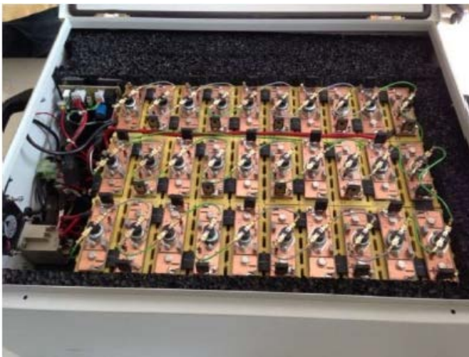
Figure 2.7 - Prototype Li-ion battery pack
