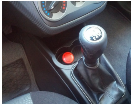
Figure 3.7 - Emergency button placement
