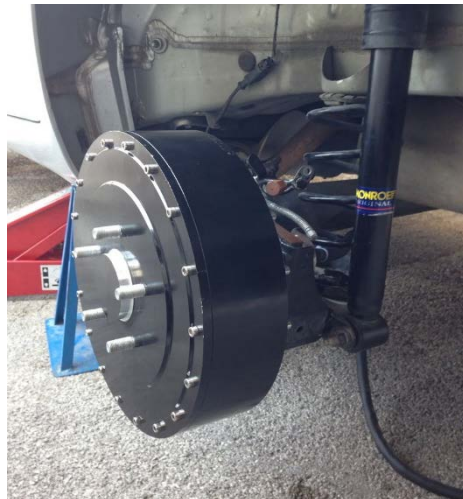
Figure 3.4 - IWM Prototype installation result
