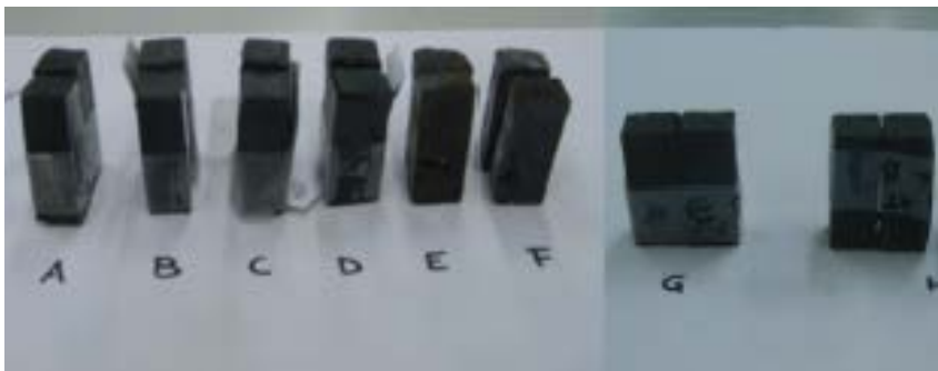
Figure 5. 5 Detail of failure of bonded joints occurred in butt joint tests.
