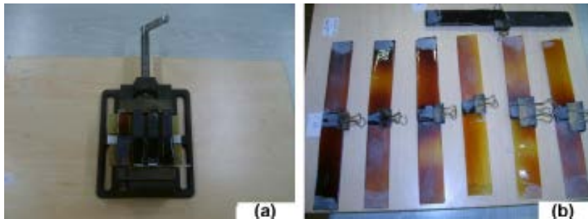
Figure 5. 4 (a) Assembly of the tensile butt joint specimens under uniform compression (before curing) and (b) assembly of the single lap joint shear specimens under uniform compression (before curing).
