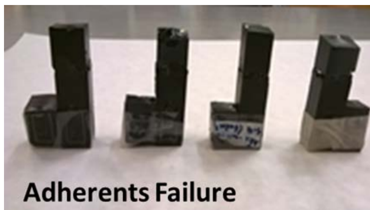
Figure 5. 22 Detail of the mechanism failure in the adherents of sample D'
