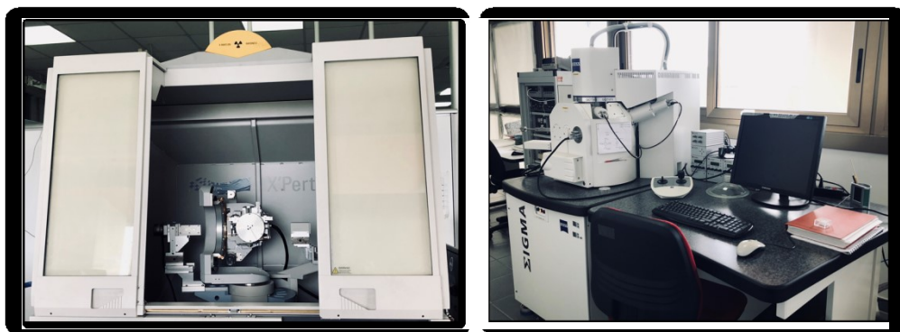
Figure 2. 11 XRD and FESEM equipment installed at MUSA lab of SPIN-CNR (U.O.S. Salerno) on the left- and right-side, respectively.
