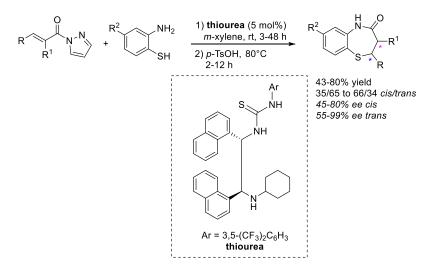
**Scheme A.** Our approach for the synthesis of *cis*- and *trans*-2,3-diaryl substituted 1,5-benzothiazepines from  $\alpha,\beta$ unsaturated *N*-acylpyrazoles.
