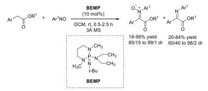
Scheme D. Synthesis of nitrones and imines through the reaction of arylacetic esters and nitrosoarenes.
