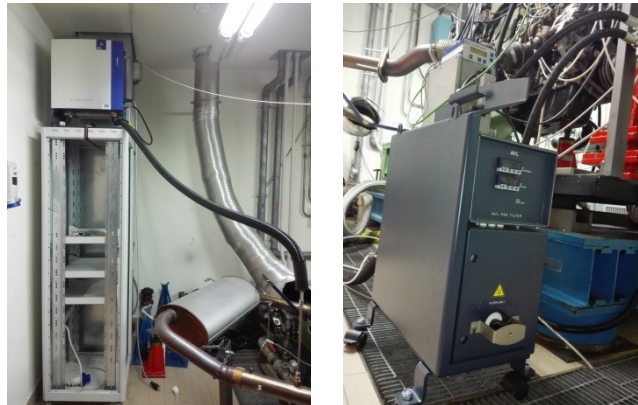
Figure 23 – AVL Smoke Meter 415S for Soot analysis (left side) and AVL pre-filter HSS i60 for Soot filtering before the gas analyzer line (right side).
