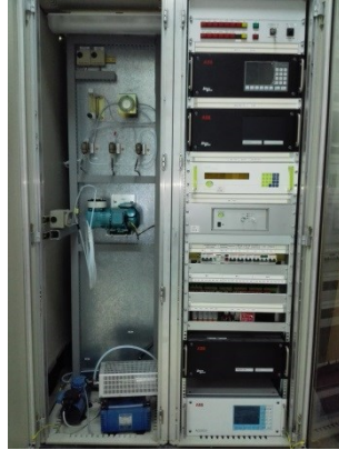
Figure 24 – Gas analyzer box. On the left side the sampling pump, on the right side the control module (Advance Optima) and the different gas modules: Uras 14, Multi-FID 14, Magnos 106 and Eco-Physics CLD700.
