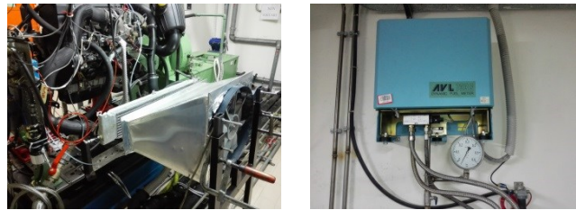
Figure 19 – Intercooler and the dedicated electric fan (left side). Dynamic Fuel Meter AVL 733S (right side).
