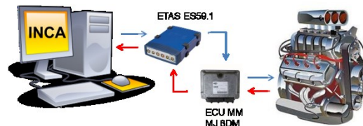
Figure 26 – Communication scheme between user and engine. Actuation line in blue: input engine variables set by the user; Acquisition line in red: feedback on control strategies from the engine.
