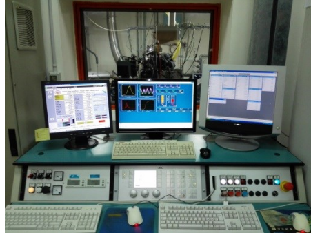
Figure 25 – The engine control console. From the monitor on the left: AVL Puma Open for the test bench sensors control; AVL Indicom v2.2 for indicating data treatment and ETAS Inca v7.0 for the management of the ECU.
