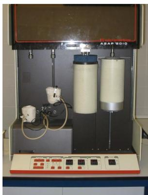
**Figure 14. Nitrogen Adsorption Porosimetry ASAP 2000 apparatus.**
