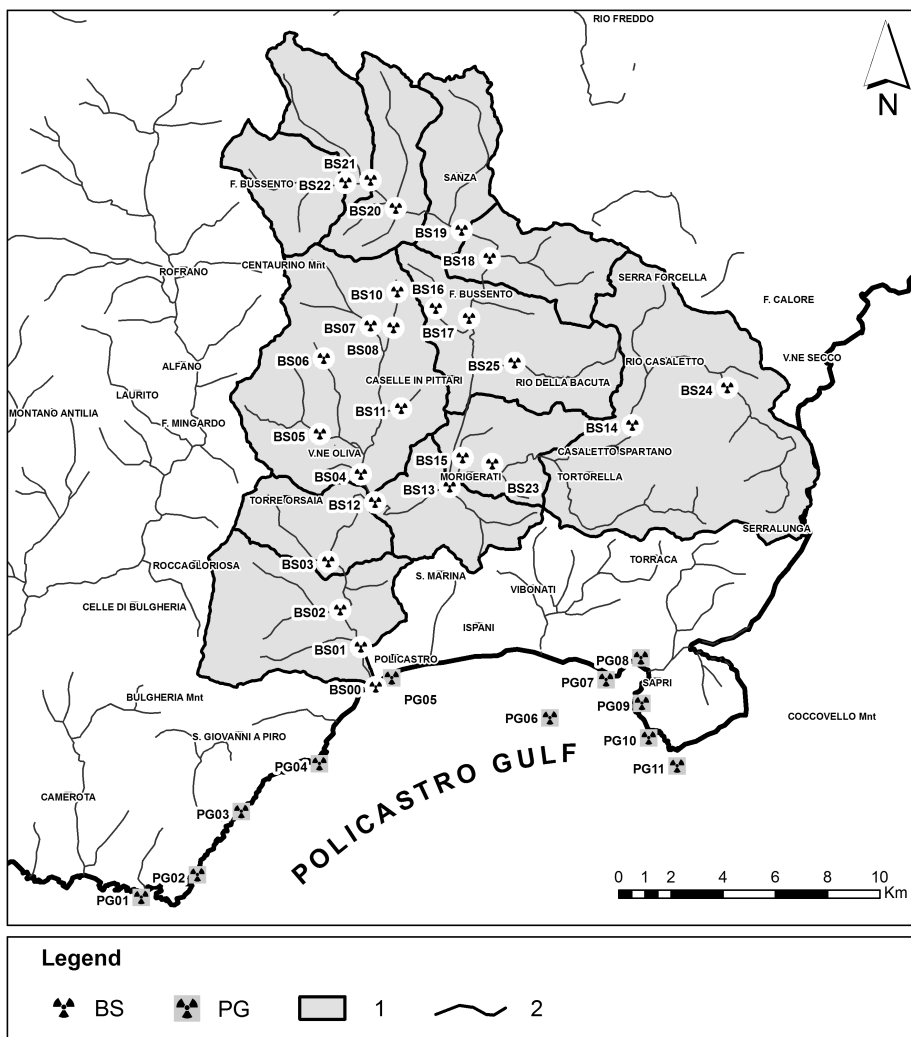
Figure 4.7: Map of the Bussento Radon Monitoring Station System (BRMSS). Legend: BS) Bussento river station; PG) Policastro gulf station; 1) Bussento river basin; 2) Watershed.
