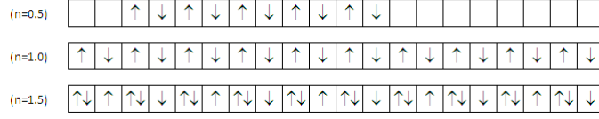
Figure 3.6: Some of the possible spin and charge configurations for the AF-phase at T = 0 , J = -1 .
