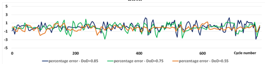
Figure 3.18 – Percentage error in results provided by neural network compared to sampled data
