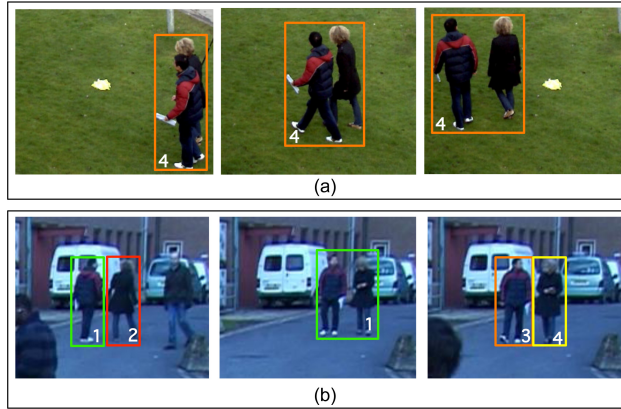
Figure 3.8 Occlusion related problems. In (a) the appearance of a group of people change from being identical to a single person to being clearly a group; if the classifier uses a classification result obtained in the first frame, it will continue to track the group considering it as an individual object. In (b) the system would not be able to correctly track the individual objects during all their life as a group if it attempts to exploit the uniformity of the motion, since the group can have strong changes in direction.
