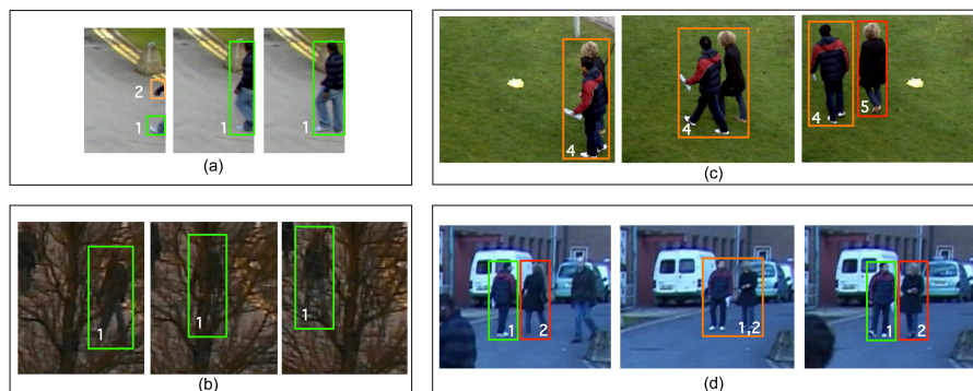
Figure 3.11 Output of the tracking algorithm based on the proposed FSA, when applied to the problems discussed in Section 3.1.2.1. (a) The entering object is correctly recognized as a single object, and not a group. (b) The object identity is preserved when the person passes behind the tree. (c) A group initially classified as a single person is correctly handled when classification becomes stable. (d) The group object maintains the constituent object identities.
