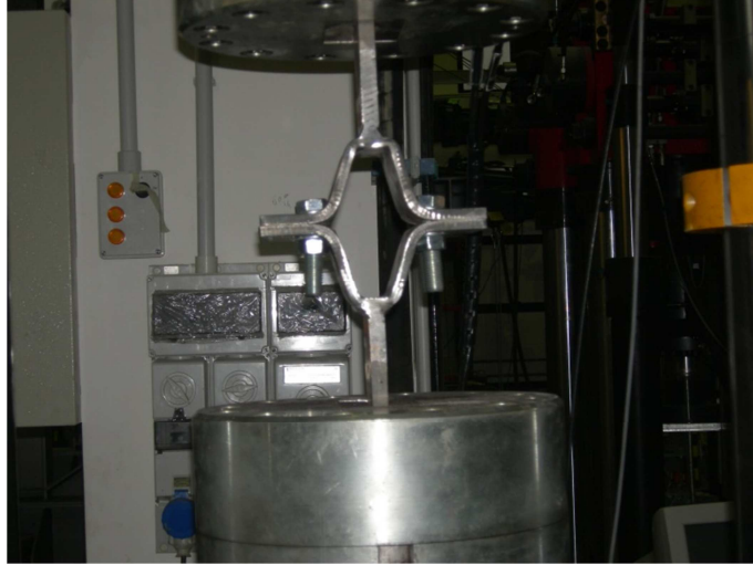
Fig. 5.51 – Typical failure of TSD specimens
