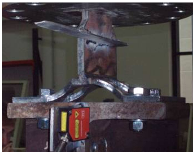
Fig. 5.38 – Experimental test on hourglass T-stub on rigid Support
