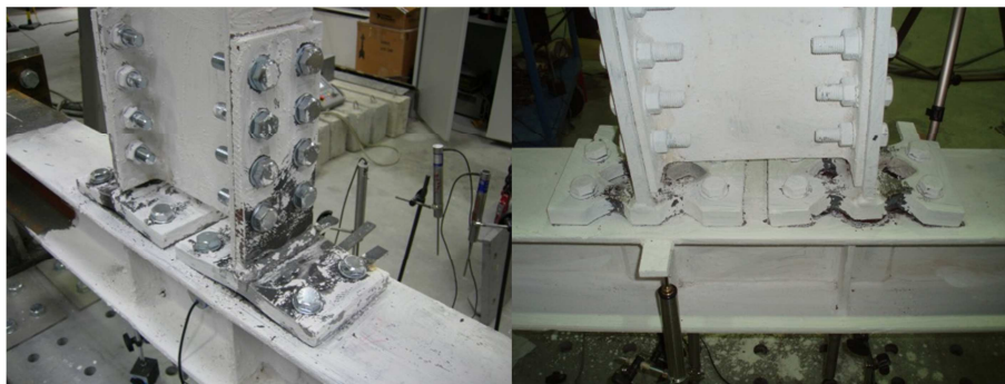
Fig. 5.79 –Joints after failure. On the left: TS-CYC-04- On the right: TS-XS-CYC-06
