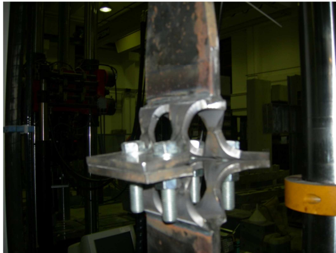
Fig. 5.52 – Typical failure of TSD-XS specimens
