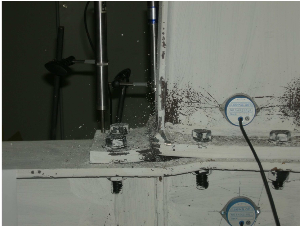
Fig. 3.37 – Failure of the end-plate
