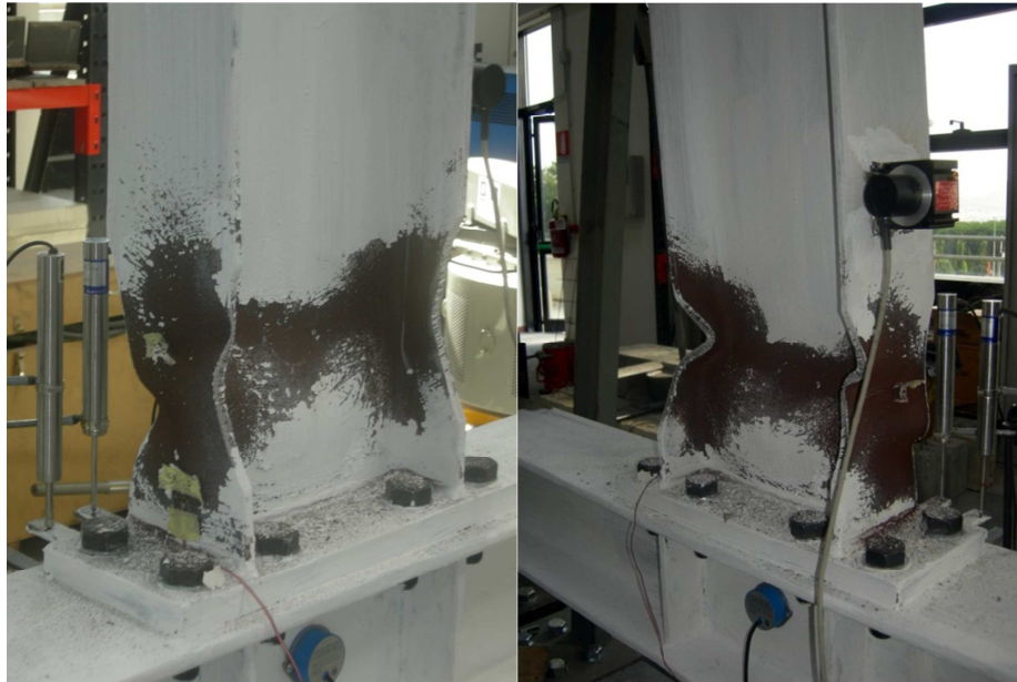
Fig. 3.43 – Flange and web buckling
