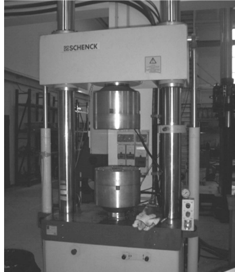
Fig. 3.3 – Universal testing machine SCHENCK Hydropuls S56
