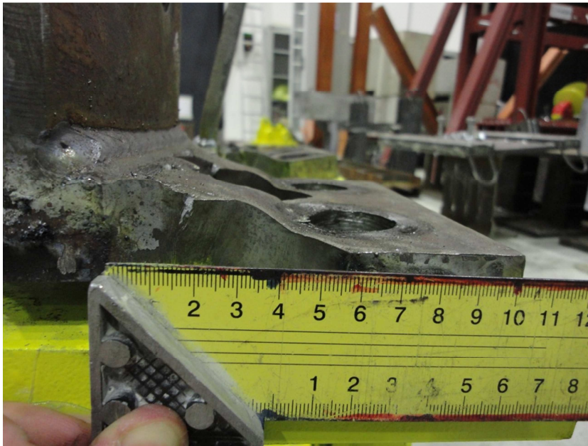
Fig. 5.86 – Position of the section of minimum resistance (TSJ-XS-CYC 07)
