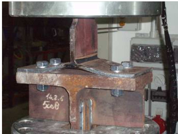
Fig. 5.39 – Experimental test on rectangular T-stub on rigid Support
